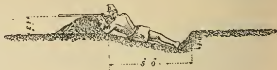
FIG. 27.—Shelter Trench,—constructed in 25 min to ½-hour
