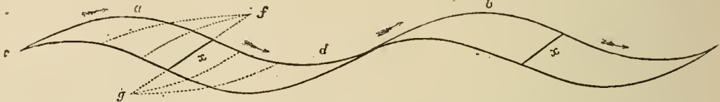
FIG. 13.—Wave track made by the wing in progressive flight. a, b, crests of the wave; c, d, e, up strokes; f, g, points corresponding to the anterior margin of the wing, and forming a centre for the downward rotation of the wing (a, b); h, i, j, point corresponding to the posterior margin of the wing, and forming a centre for the upward rotation of the wing (d, e). (Pettigrew, 1867.)
