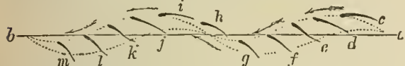
FIG. 30 shows the kite-like action of the wing during the down and up strokes how the angles made by the wing with the horizon (a, b) vary at every stage of these strokes, and how the wing evades the superimposed air during the up stroke, and seizes the nether air during the down stroke. In this figure the spaces between the double dotted lines (a, g, i, b) represent the down strokes, the single dotted line (h, i) representing the up stroke. The kite-like surfaces and angles made by the wing with the horizon (a, b) during the down strokes are indicated at c, d, e, f, g, j, k, l, m,—those made during the up strokes being indicated at g, h, i. As the down and up strokes run into each other, and the convex surface of the wing is always directed upwards and the concave surface downwards, it follows that the upper surface of the wing evades in a great measure the upper air, while the under surface seizes the nether air. It is easy to understand from this figure how the wing always flying forwards furnishes a persistent buoyancy. (Pettigrew, 1870.)
