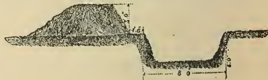
FIG. 30.—Shelter Trench,—3½ hours.
