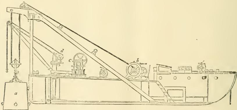
FIG. 4.—Longitudinal Section of Diving Bell Lighter (56 feet long and 21 feet beam).
