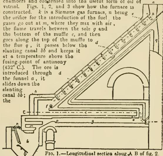
FIG. 1.—Longitudinal section along A B of fig. 2.
