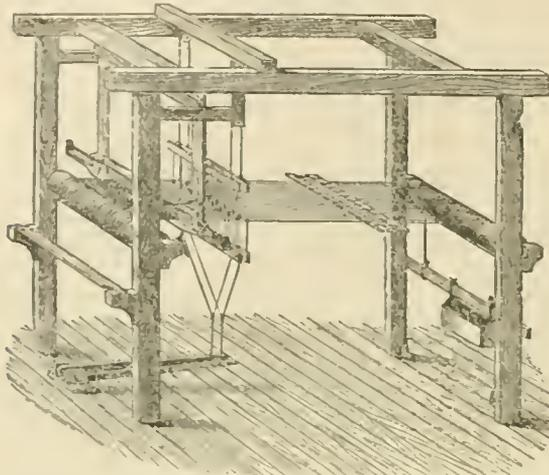
FIG. 1.—Diagram of Hand-Loom.
