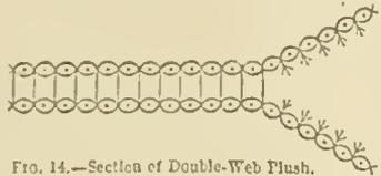
FIG. 14.—Section of Double-Web Plush.
