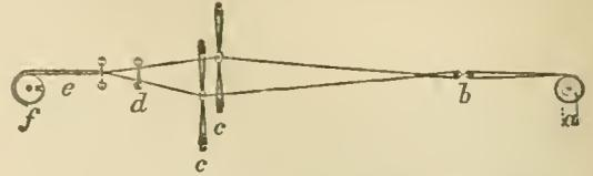
FIG. 3.—Section of plain web in process of weaving on the loom: a, warp beam; b, leash rods where the warp is divided and crossed; c, c, heddles; d, reed; e, the woven cloth; f, the cloth beam.
