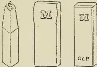
FIG. 2.—Punch. FIG. 3.—Drive. FIG. 4.—Matrix.
