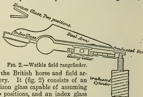
FIG. 2.—Watkin field rangefinder.
