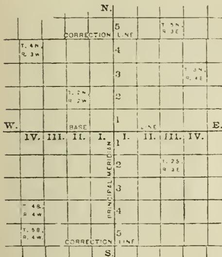
measure from some selected point, marking each half-mile point with a "quarter stake," and each mile point with a "section corner." At each six-mile point a "township corner" is marked. This line is called a *principal meridian*.
