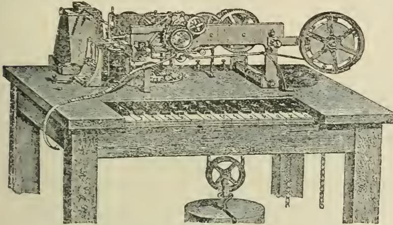
FIG. 19.—Hughes's type-printing instrument, one-tenth full size.
