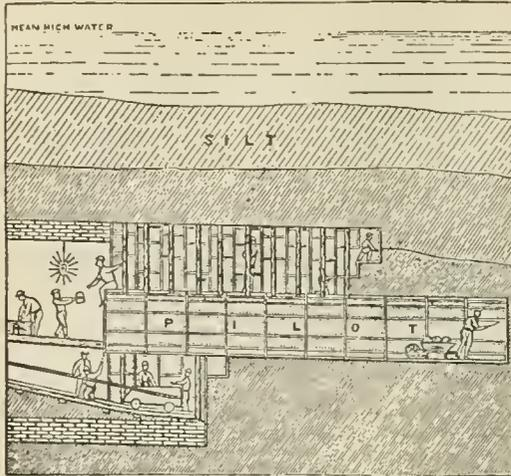
FIG. 2.—Hudson river tunnel—method of work.
