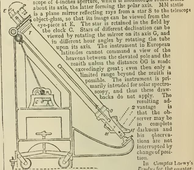
FIG. 31.—Grubb's siderostatic telescope.
