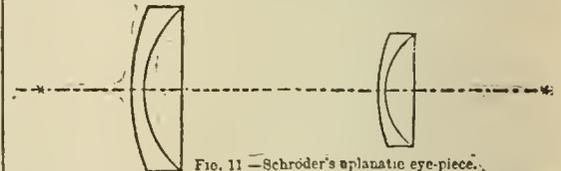
FIG. 11.—Schroder's applanatic eye-piece.
