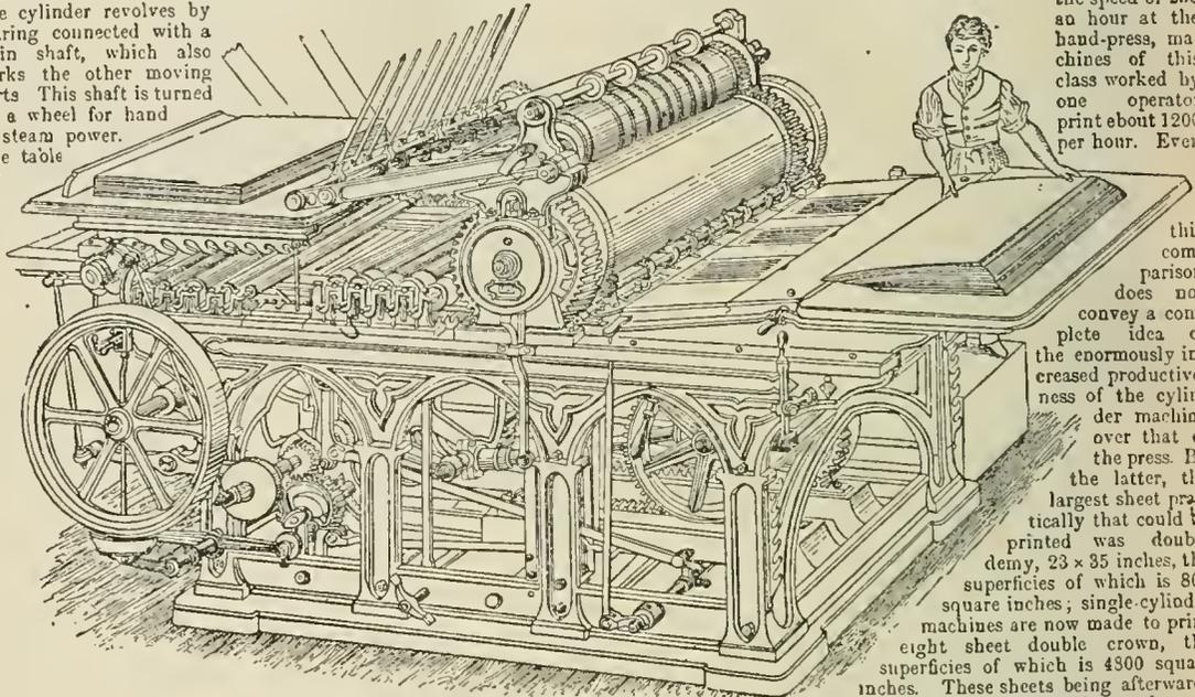
FIG. 12 — Extra colour Bremner machine, with sheet-flyers.
