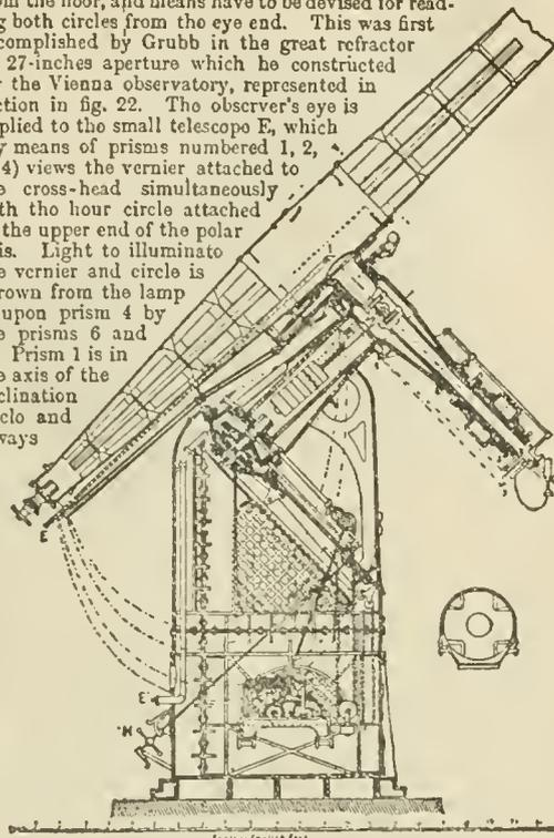
FIG. 22.—Grubb's 27-inch refractor (Vienna).
