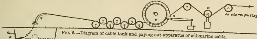
FIG. 6.—Diagram of cable tank and paying out apparatus of submarine cable.
