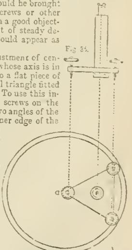
FIGS. 35, 36.—Apparatus for adjustment of centring in a small telescope.
