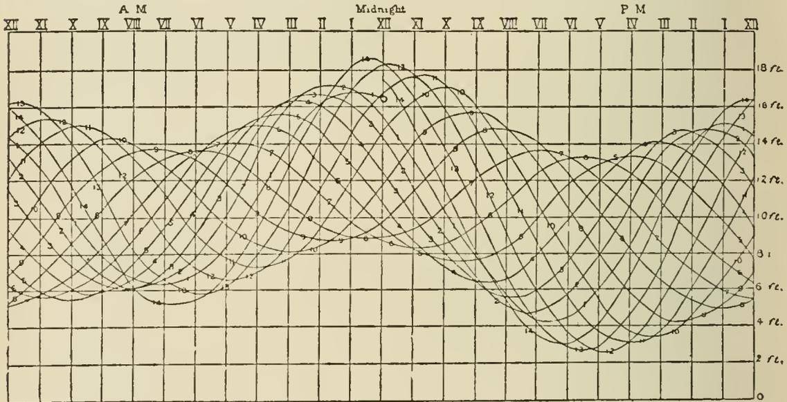
FIG. 3.—Tide-curve for Bombay from the beginning of the civil year 1834 to the midnight ending Jan. 14, 1834, or from 12h Dec. 31, 1833, to 12h Jan. 14, 1834, astronomical time.
