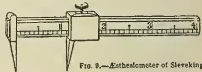
FIG. 9.—Aesthesiometer of Sieveking.
