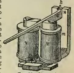
Fig. 25.—Siemens's polarized relay.
