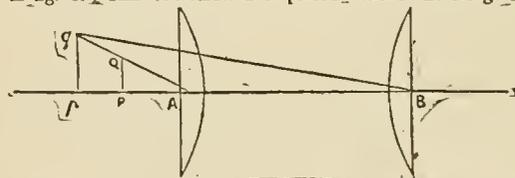
FIG. 8.—Common or positive eye-piece.
