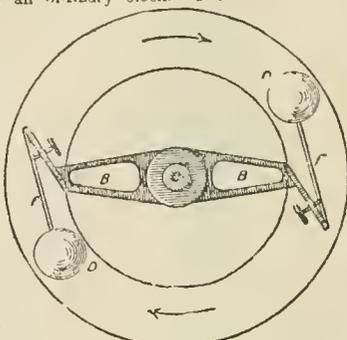
FIG 37.—Fraunhofer's governor
