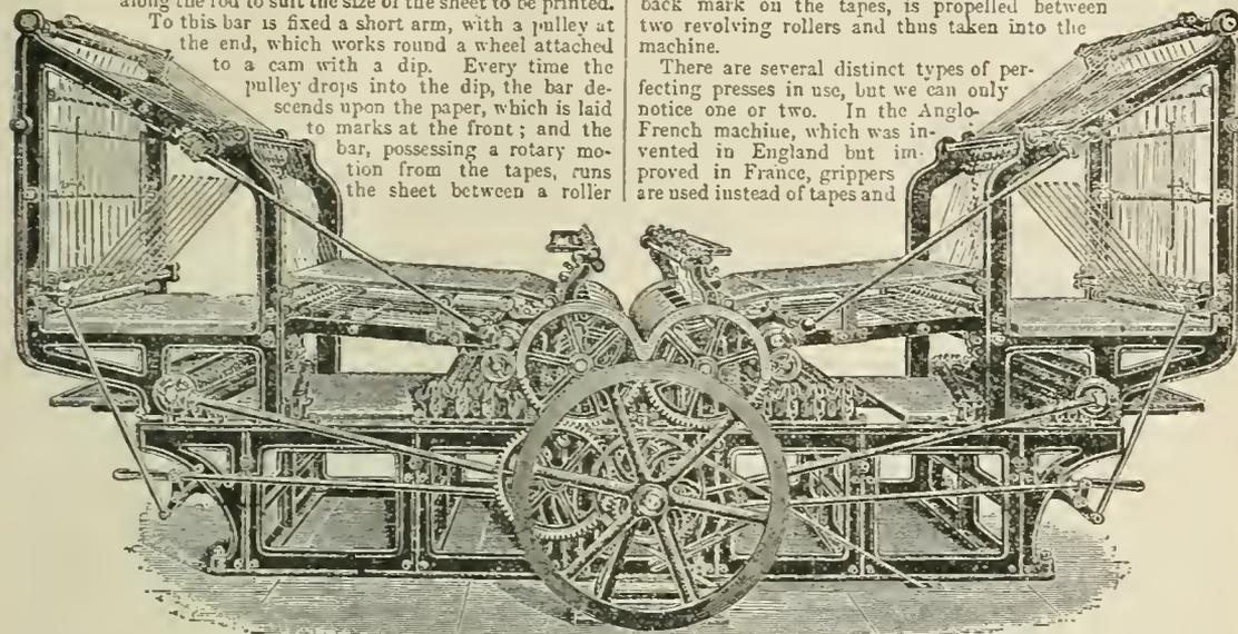
FIG. 13.—Marioni combined perfecting and duplex single-cylinder machine.
