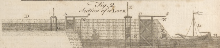
Fig. 3. Section of a Lock full of Water
