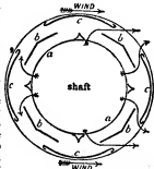
FIG. 4.—Sectional Plan of Buchan's Exhaust Cowl.
