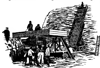
FIG. 2.—Thrashing Machine at work with stacking elevator behind. (Clayton & Shuttleworth, Lincoln.)
