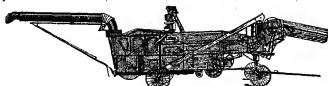
FIG. 4.—American "Separator" with self-feeder and fan-blast delivery-pipe for straw. (Avery Manufacturing Co., Peoria, Illinois.)
