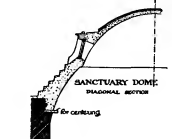
Fig. 14.—Westminster Cathedral: diagonal section through sanctuary dome.
