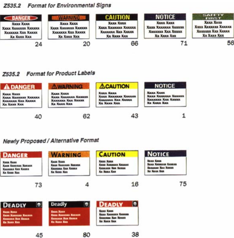
Figure 7.2 ANSI Z535.2 (environmental signs), ANSI Z535.4 (product labels), and alternative set of warnings tested by Wogalter et al. (1998). Used with permission from John Wiley & Sons.
