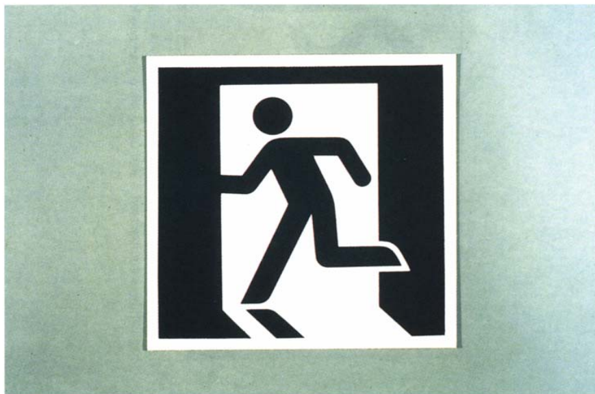
Figure 12.10 Symbol tested by NBS/NIST researchers for 'exit' that was found to communicate the message effectively and be visible in simulated smoke conditions.
