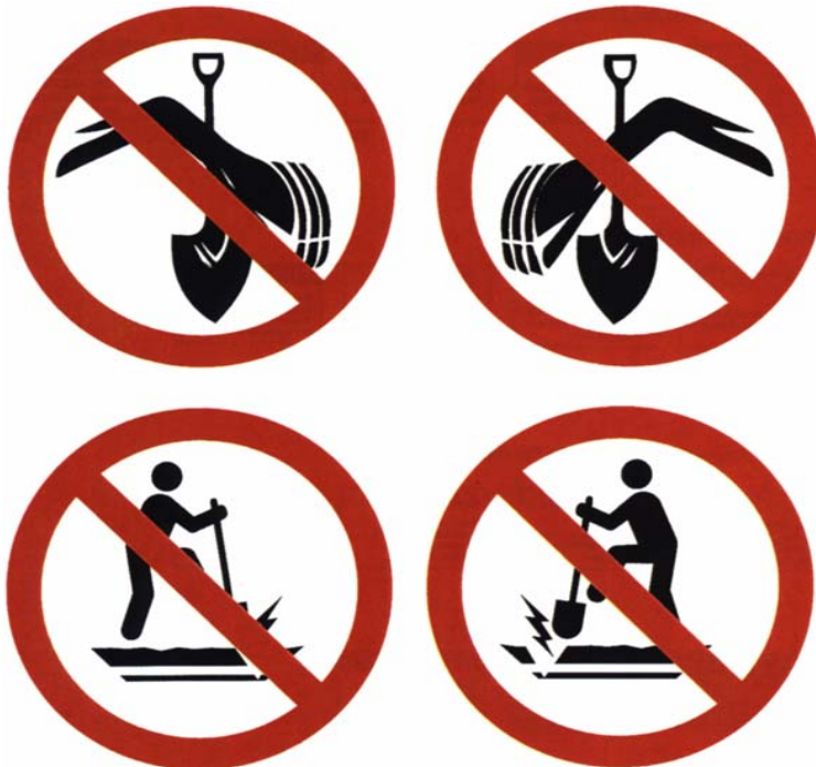
Figure 7.6 The over slash can obscure the critical parts of the internal portion of the symbol. Sometimes flipping a nonsymmetric symbol horizontally may help.
