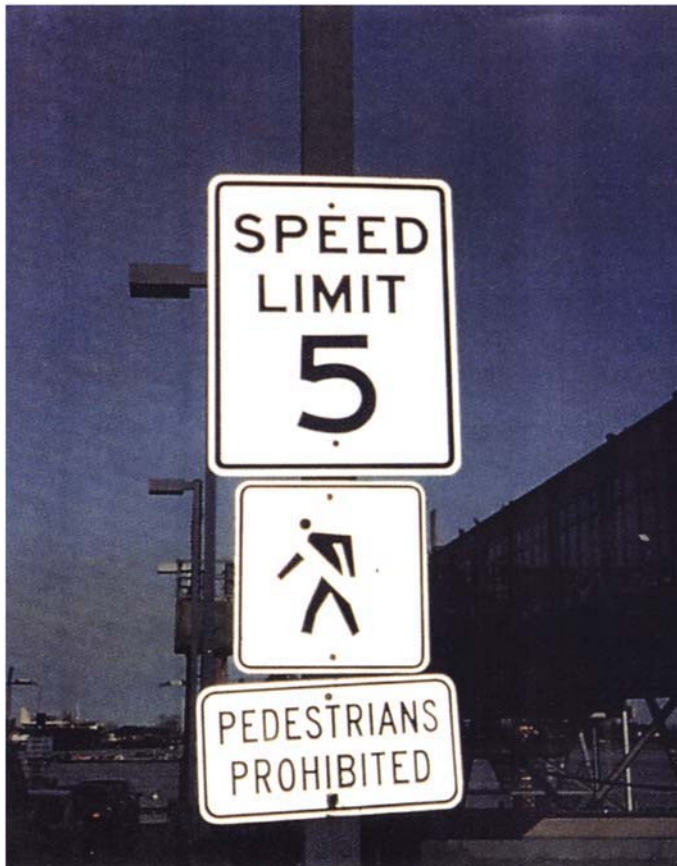
Figure 7.7 The red of the circle/slash negation symbol has faded in this sign. The two adjacent signs help to avoid a potentially dangerous critical confusion.
