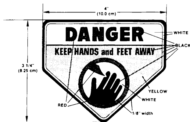
Figure 12.6 Guidelines for the design of symbols to be used on reel-type mowing machines as prescribed by the US Consumer Product Safety Commission (CPSC).
