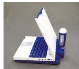
► Prototype of a laptop computer with a DMFC as its power supply: The methanol cartridge is applied only during refill processes. Fuel cells are ideal for telecommunications systems, as they permit long, uninterrupted operation of electronic devices. Source: NEC Corporation
