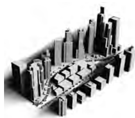
📍 Design analysis: At the beginning of a planning process, design variations are used for shading analyses, to investigate the basic problems of solar radiation in streets and buildings. Source: WSGreen-Technologies
