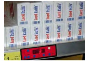
► Pick-by-light system: A display shows the picker the quantities to be retrieved for a specific consignment.
