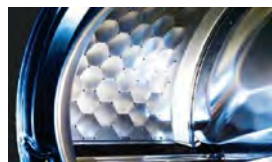
🔍 Hive-like vault structure illustrated by a washing machine tub: A hexagonal vault structure was developed here. This is an evolution from the square structure, because it achieves torsion stiffness in all directions. Source: Miele
