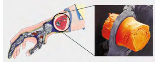
▣ Cyberhand. Left: Inside the hand prosthesis, small engines respond to instructions from the brain. Sensors at the fingertips make palpation feelings possible. In contrast to standard hand prostheses, the cyberhand uses filament electrodes implanted into the lower arm and directly attached to the nerves. Right: The connection between a nerve fibre bundle (orange) and a sieve electrode (grey). Source: Fraunhofer IBMT
