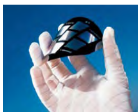
Thin-film solar cell: This crystalline silicon cell demonstrated that wafers with a thickness of 30 \mu\text{m} are sufficient to produce solar cells with efficiency values exceeding 20%. Source: Fraunhofer ISE
