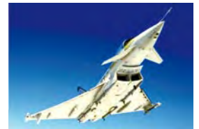
■ Eurofighter: The additional control surface at the front, known as a canard wing, gives this fighter aircraft greater agility. Source: Refuelling Ltd.
