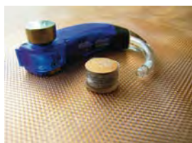
► Small scale application of a lithium ion battery: The cell has a capacity of 15 mAh and 3.7 V. It is used in hearing aids and delivers electricity for one day.
