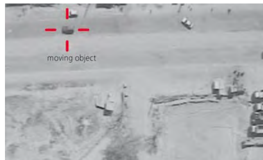
► Detection of moving objects: A moving car that has been recorded in a video sequence from a fast flying aircraft is detected and marked. The detection is based on features that are characteristic for a moving car, such as its proper dynamics in the motion-compensated image sequence, or its dimensions and shape. Source: Fraunhofer IITB
