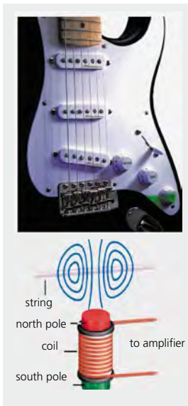
📌 Electric guitar. Top: 3 rows of magnetic single coil pickups are mounted at different locations between the bridge (bottom) and the neck (top) of the body. The switch (right) lets the musician select various combinations of the three pickup devices. 3 rotary knobs drive active filter/amplifier circuits to change the volume and timbre of the sound. Bottom: Magnetic guitar pickup. An alternating current is induced in the coil by the magnetic field of a vibrating steel string. Source: Fender® Musical Instruments
