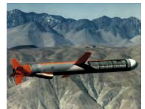
► Tomahawk cruise missile in action: The major components of this cruise missile are (from front to back) detector head, navigation system, warhead, fuel tank, navigational computer and jet engine. Source: Raytheon
