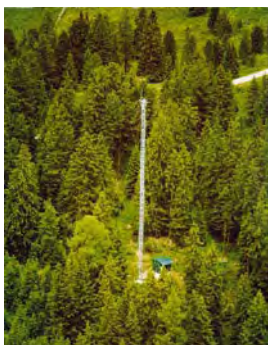
■ Micrometeorological eddy covariance tower in Italy (viewed from the air): The exchange of air packets between the forest and the lower atmosphere is measured at frequent intervals and a balance is calculated. This determines whether a forest is actually storing the quantity of carbon specified as the target value by a forestation project. Source: Forest Department of the Autonomous Province Bolzano/Bozen Minerbi
