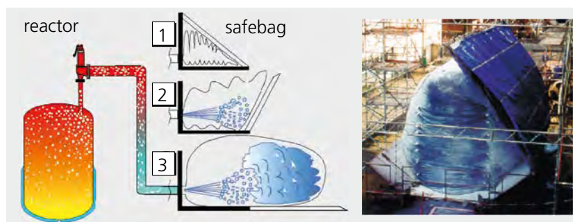
► Pressure is released in a controlled way through safety valves into safety bags to prevent any substance leakage. The bags are made of chemical-resistant, coated material and are used, amongst other things, to render boilers or distillation columns safe. They take up almost no space when empty. Left: An empty safebag (1), at the beginning (2) and towards the end (3) of a pressure release cycle. Right: A safebag after pressure has been released. Source: Siemens Axiva GmbH
