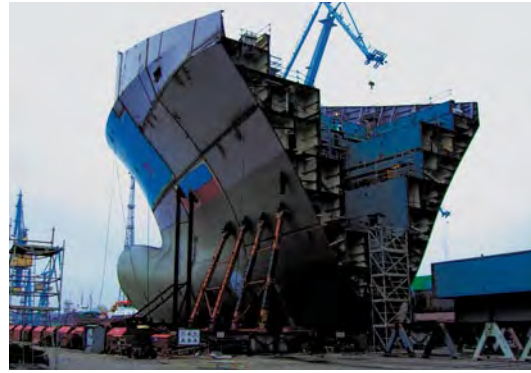
3 Bow section of a fast containership built on keel blocks: In shipbuilding today, the individual sections are pre-fabricated and then assembled to form the ship's body. Thanks to a system of rails, the ship can be moved about the shipyard according to work requirements. Source: Fraunhofer AGP
