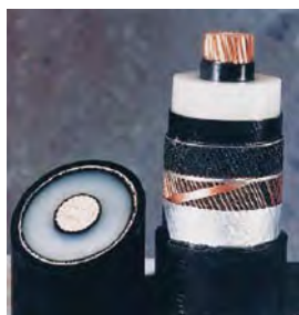
☑ Cross-section of a high-voltage cable. From center to rim: conductor, insulation, mechanical protection layer made of steel armor and plastic. Source: Arbeitskreis Schulinformation Energie
