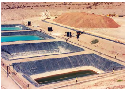
🔍 Bioleaching of heaps: Collecting ponds can be seen in the lower and upper left-hand corners. In the upper right-hand corner, a 1,000-t heap is piled up for percolation leaching using an alkali-sealed leaching pad. The heap is sprinkled with the acidic leaching agent containing the bacteria. The solution is enriched with metals and then drains into the collection ponds by gravity. The blue colour of the leachate in the upper collection pond indicates the presence of copper sulphate. Source: BGR
