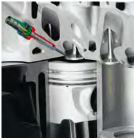
❑ Glow plug with integrated pressure sensor: The glow plug descends directly into the combustion chamber and the pressure exerted on the sensor (green) is used to regulate the temperature of the glow plug and hence the timing of the ignition of the fuel-gas mixture. Source: Bern AG
