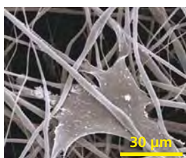
Cell cultured on a nanostructured plastic surface under investigation as an implant material: Cell cultures are grown on nanomaterials to investigate the effect of nanostructures on the adhesion, growth and reproduction of cells. Source: Dr Dalby, University of Glasgow
