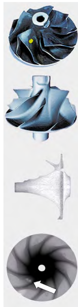
❏ High-resolution CT of a turbine rotor showing a casting flaw. From top to bottom: Optical view, 3D volume reconstruction, 2D slice through 3D data set and single radiograph. The casting flaw is indicated. Source: Viscom AG
