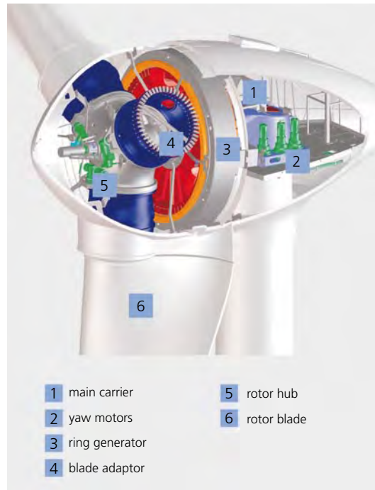
▣ Nacelle of a 2 MW wind turbine: The blade adapter connecting the rotor blades with the hub permits active adjustment of the rotor blades to set an optimum angle of attack. In this model, the rotor hub and the ring generator are directly affixed to each other without a gear box. Output voltage and frequency vary according to speed and are converted for transfer to the power grid via a DC link and an AC converter. This permits high speed variability. Yaw control is provided by the horizontally rotating yaw motor. Source: Enercon GmbH
