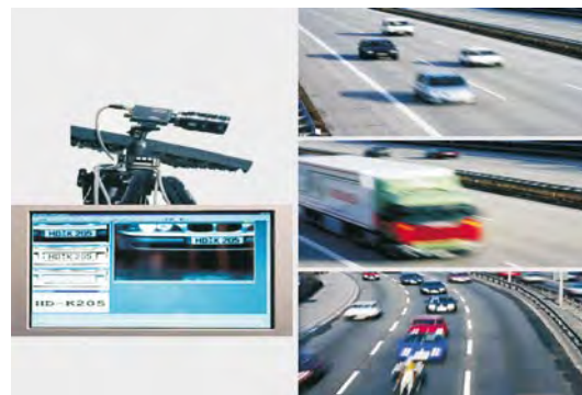
License plate recognition: Image analysis methods are used to detect the license plate in the recordings of passing vehicles and to identify them using optical character recognition (OCR). Source: Fraunhofer IGD
