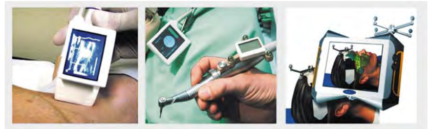
■ Integrated monitors. Left: Ultrasound device with integrated monitor. While image data are recorded, they are visible directly on the ultrasound head at the same time. Centre: Small monitors for instrument navigation, which can be attached directly to or in the operation area. The monitors can be much smaller, without any loss of information, as the distance to the eye is less. If a monitor’s position in the area is known, it displays information relative to the situation, e.g. anatomical descriptions. Right: Navigated image viewer with reverse camera. The monitor makes it possible to carry out a review, with relevant 3D patient images superimposed in the exact position. It is almost like being able to see inside the patient. Source: T. Lüth
