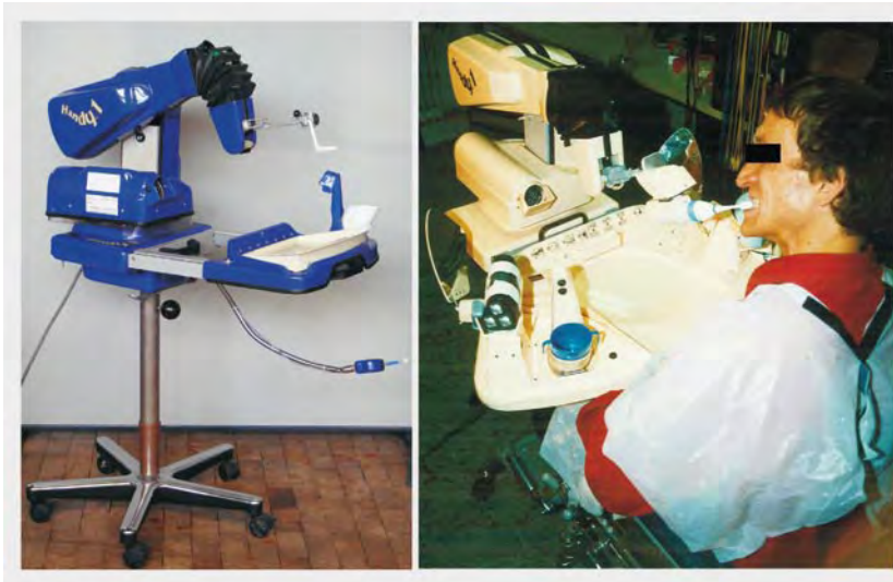
▣ Rehabilitation robot: The robot consists of a simple 5-axis arm and a set of exchangeable, automatically detectable application trays, e.g. one for “meals” with a dish, spoon and cup (left) or one for “personal hygiene” with a water bowl, soap, sponge, electric shaver, electric tooth brush, water cup, and mirrors. The basic equipment includes an electric fan for users to dry their face. Each tray has a set of predefined robot functions which are sequentially displayed with LEDs and can be activated through a single switch. This allows even severely physically disabled people to control the robot.
