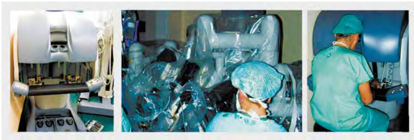
Operating console of a telemanipulator. Left: The foot switches and the “joysticks” for the hands can be seen, together with the two circular openings for viewing the stereo monitor. Centre: The robot itself has three arms – one for the endoscope and two for the instruments. The arms are sealed in special plastic bags to keep them sterile. The sterilised instruments are introduced via small incisions in the body. This is inflated with nitrogen gas, so that the surgeon can work in the cavity. Right: The surgeon sits at the console a few metres away from the patient and moves the instruments in the body. Source: T. Lüth
