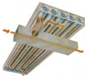
❏ Thermally activated building components: A hot or cold medium (air or water) is pumped through a serpentine array of tubes integrated in the building component, heating or cooling the room according to the selected operating mode. The high thermal mass of the concrete ensures a more or less constant ambient temperature, even when no air or water is being pumped through it. Source: Fraunhofer IBP
