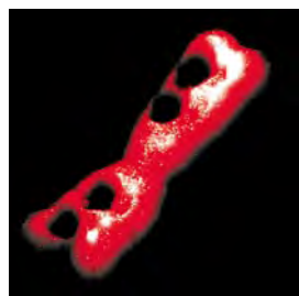
Nanosurgery with femtosecond lasers: Nanoholes with a diameter of less than 100 nm in a human chromosome are depicted.
