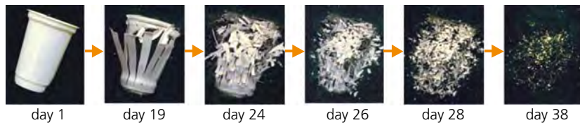
Biodegradation of bioplastics: In the composting plant, a cup is completely decomposed by microorganisms within about 5 weeks.
