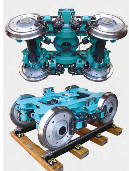
► Leila (light and low-noise) with crosslinks for radial steering. Top: View from below. Bottom: Overall view. The crosslink equalises the steering of the leading and the trailing axles and stabilises movement at high speed. Apart from improving energy efficiency, this bogie also reduces noise significantly thanks to a special low-noise wheel design, damping in the high-frequency range with rubber springs and hydraulic instead of friction damping. Reliability is also improved over conventional designs by reducing the number of friction surfaces. Source: Josef-Meyer Transportation
