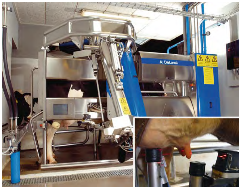
► Automatic milking system (“milking robot”): The entire milking process takes place automatically without the presence of personnel. Inset: Automatic attachment of the teat cups. A laser-assisted image processing system locates the position of the teat. Source: DeLaval GmbH, Sweden
