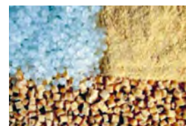
► WPC granules: The two main components of WPC are polyethylene and wood flour. Source: USDA
