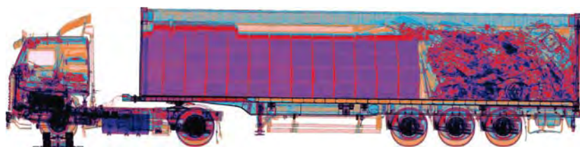
■ X-rayed lorry: Goods smuggled in lorries and transport containers are often hidden behind several tonnes of camouflage goods. A customs officer without an X-ray image at his or her disposal is very unlikely to have found the 4 million cigarettes in the lorry, which can be clearly seen on the image. Source: Smiths-Heimann
