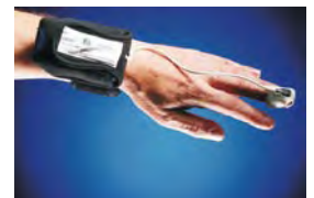
■ OxiSENS: Wireless pulsoximeter for measuring oxygen saturation on the finger. Source: Fraunhofer IIS
