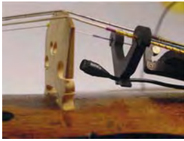
▶ Miniature microphones for live applications: To pick up string instruments in live applications, miniature microphones like this one are applied to reinforce the sound of the instrument. Source: DPA Microphones A/S
