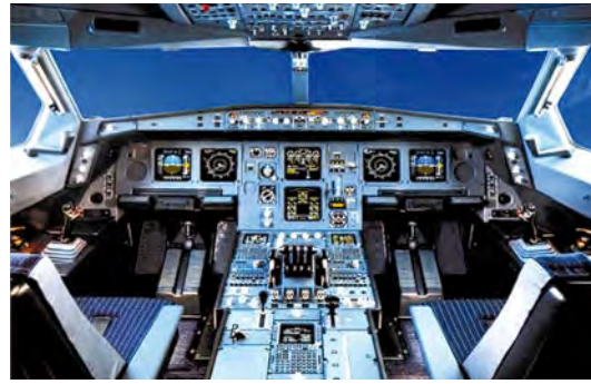
▣ Cockpit of an Airbus A340: The arrangement of instruments in the cockpits of large transport aircraft, even in different models, is very similar. However, the in-flight behaviour of different aircraft types can vary widely. Electronic flight control can overcome these differences, so that pilots need less familiarisation time when flying different aircraft types. Source: Airbus
