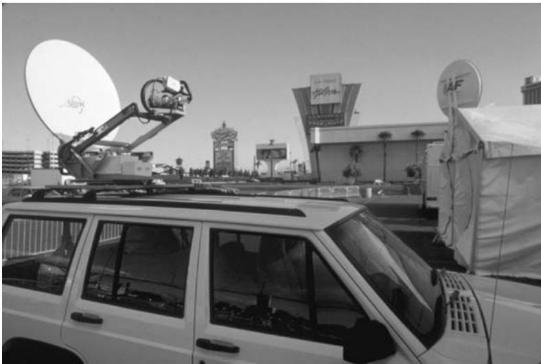
Figure 6.5 An SNG vehicle. Note the portable dish size. (Courtesy of Intelsat.)
