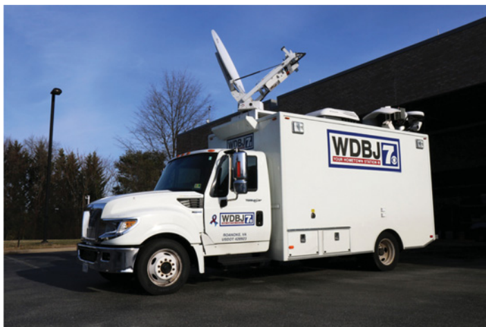
Figure 10.13b Satellite truck used by the WDBJ television station in Roanoke, Virginia, for outside broadcasts. The main satellite communication antenna is shown in its operating position. Source: Photographs courtesy of WDBJ-TV, © WDBJ-TV 2018.
