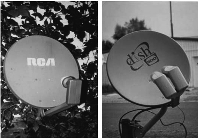
Figure B.5 Early design of DBS-TV receiving antenna with a circular aperture and a single feed (left) and a dual feed (right). Photo credit: Tim Pratt.
