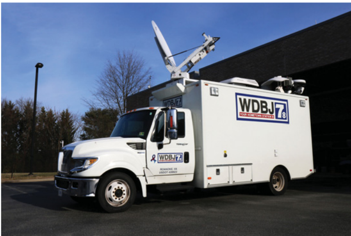
Figure 10.13b Satellite truck used by the WDBJ television station in Roanoke, Virginia, for outside broadcasts. The main satellite communication antenna is shown in its operating position. Source: Photographs courtesy of WDBJ-TV, © WDBJ-TV 2018. For a color version of this figure please see color plate section.
