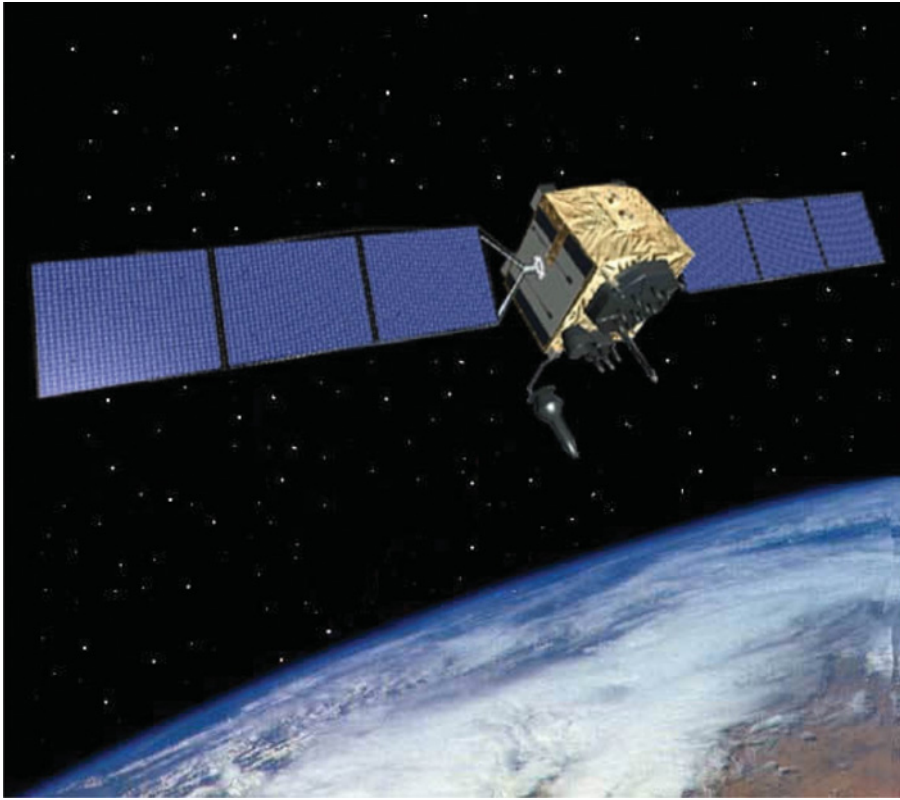
Figure 12.1 Block IIF GPS satellite. Source: US government. For a color version of this figure please see color plate section.
