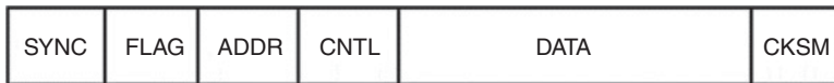
Figure 5.16 Generic packet structure. The SYNC block is used to synchronize the bit clock in the receiver, FLAG (or a unique word) indicates the start of the packet, ADDR is where the transmitter and receiver addresses can be inserted, if needed, and CNTL is where control bits are inserted. The DATA block can be of fixed length, or variable length in which case the number of data bits will be given in CNTL. CKSM is a checksum used by the receiver to verify that errors have not occurred in the packet. Frequently, a cyclic redundancy check (CRC) is used in preference to a checksum because a CRC can find multiple errors in a packet.
