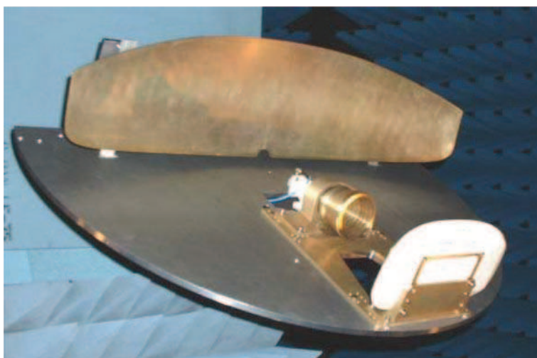
Fig. 6. A prototype antenna suitable for the pendolino trains (courtesy of teleinformatica& sistemi – patent pending).
