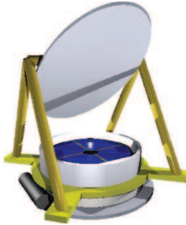
Fig. 7. Artist's view of the combined microwave-optical ILS terminal for microsattellites.
