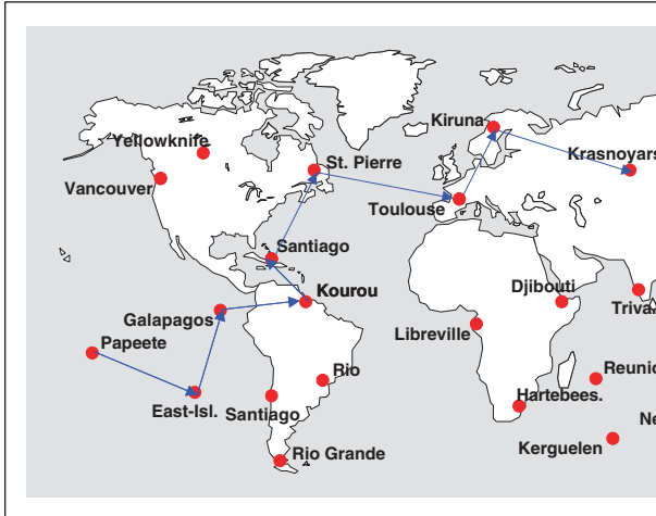
Fig. 4. Example of linked common-view time transfer.
