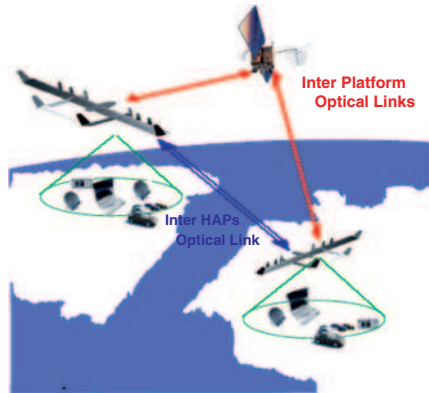
Fig. 1. HAP-Satellite link scenario: by integration of optical and RF technologies it is possible to enhance system performance.
