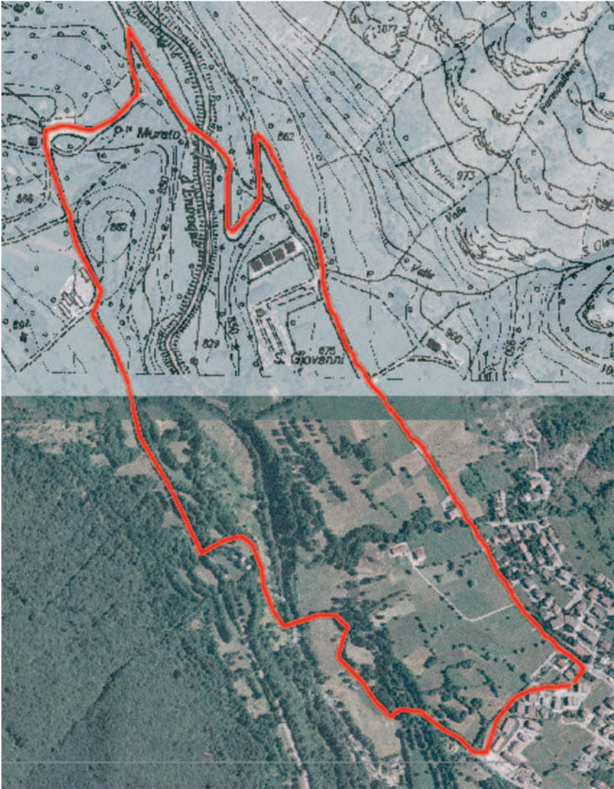
Fig. 8. Dynamic test result. The bold line represents the track of a rescuer equipped with the ISMB test prototype. This test has been conducted in a mountain environment; in particular in this area there are frequent lacks in the GPRS availability; therefore the main communication channel used for this test is VHF.
