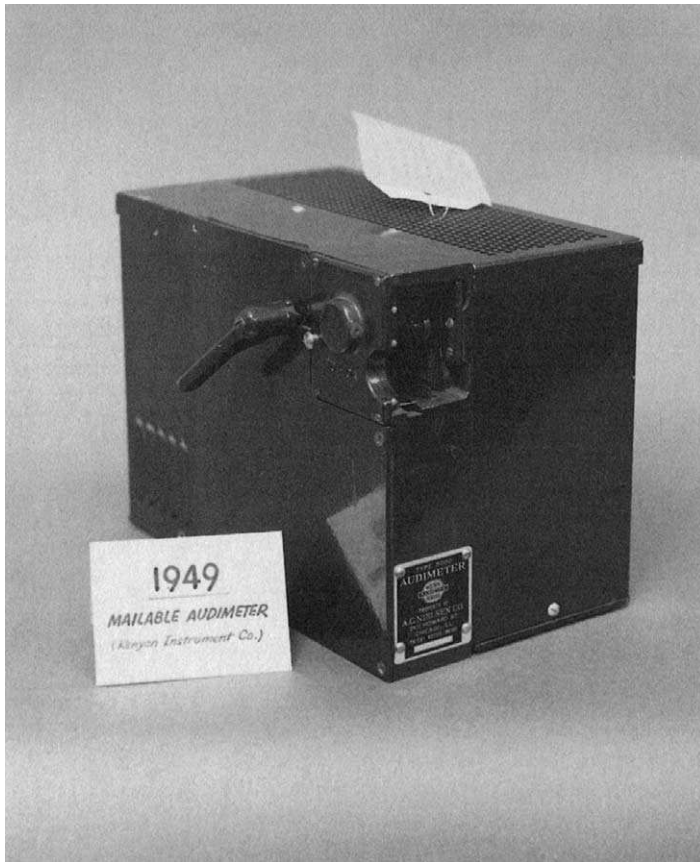
Figure 11.1 This 1949 audimeter is one of the first that could be operated without a technician's assistance. People in the survey could remove a tape and mail it to Nielsen. (Courtesy Nielsen Media Research.)
