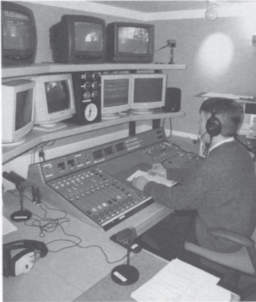
8: News Direct's on-air studio with only one person managing the station's entire output. Complete self-drive news broadcasting is achieved by a purpose-built studio integrated into text and sound editing computer storage systems. The on-air microphone is connected to the headphones giving the presenter mobility within the studio.
