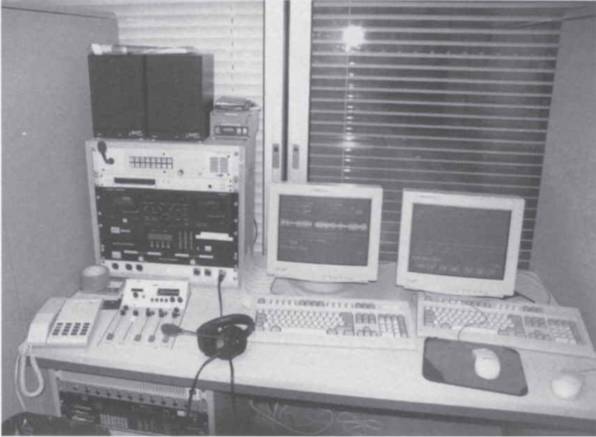
6: News Direct's intake station. Computer digital systems receive reports and outside broadcast sources by ISDN lines. Radio news communication remains digital from the point of origination all the way through to transmission.
