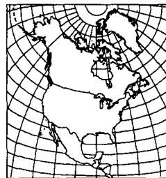
As the area becomes larger, parallels and meridians frequently appear as gently curving lines.
