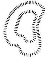
Example of hachures which were used to indicate changes in elevation before contour lines became widely used
