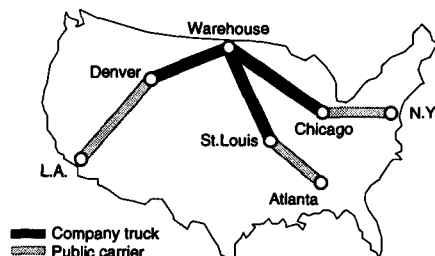
Example of a flow map including information about responsibility for different parts of flow
