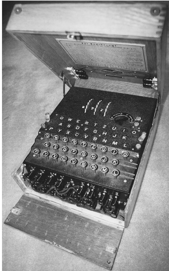
FIGURE 11.6 The Enigma machine. The machine has typewriter keys for entry, three rotors to define a letter substitution, a plugboard to implement a further substitution, and finally, lightbulbs to indicate the result.
