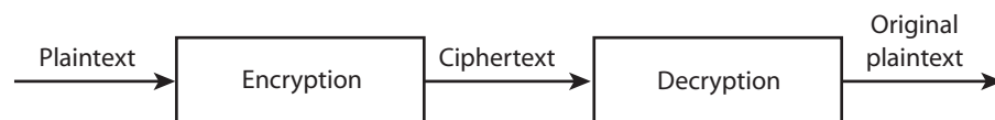
FIGURE 11.1 Cipher process. Plaintext is encrypted into ciphertext, and this is sent to the receiver, who decrypts it to recover the original plaintext.
