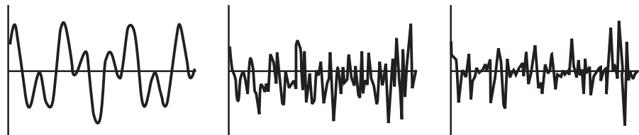
FIGURE 21.9 Spreading a signal. The first graph shows a low-bandwidth signal. The second graph shows a broad bandwidth random waveform. The third graph shows the result of multiplying the two together. The result is again essentially random with a broad bandwidth. The original signal can be recovered by dividing out the random waveform.
