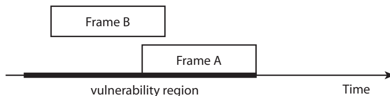
FIGURE 22.3 Vulnerability region. The vulnerability region is twice the duration of a single frame.
