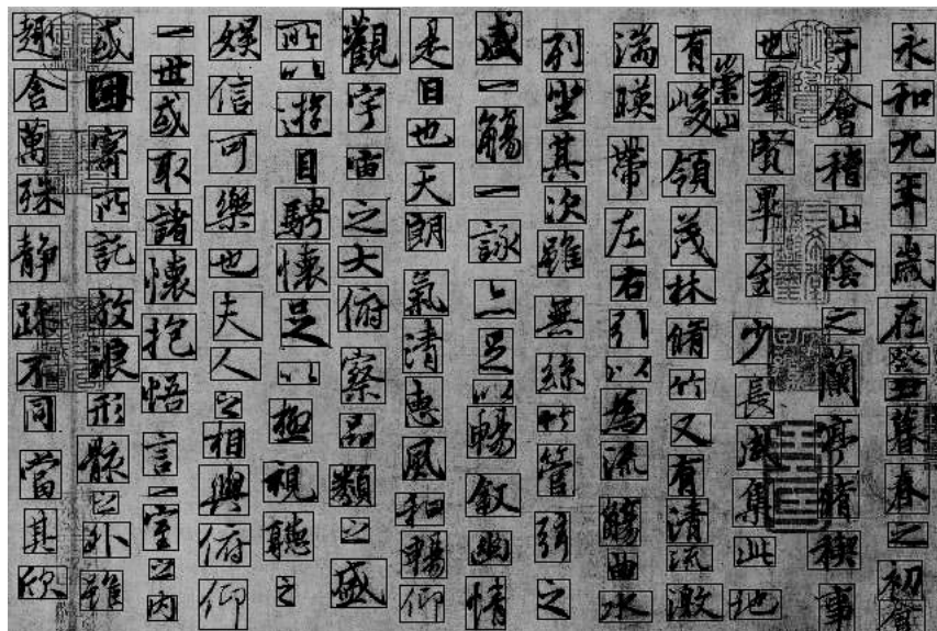
Figure 2. An example of segmenting a page into individual characters using minimum-bounding box
