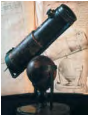
Newton's reflecting telescope, made in 1668.
