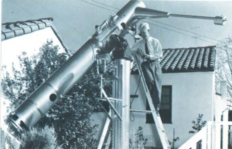
For a serious amateur: This homemade 12-inch reflector, equipped with a camera, can give high performance. ( Clarence P. Custer, M.D. )
