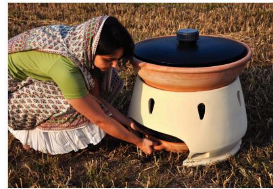
▲ Another use of solar power: making water safe to drink. River water is poured into the top container, where it's boiled by solar power. (The lid has solar cells.) The steam condenses to give clean water in the lower container.
