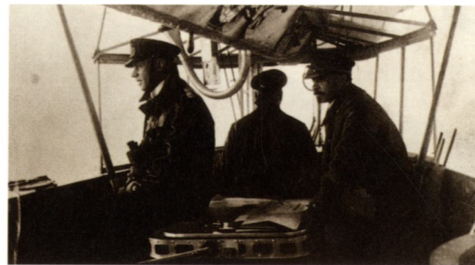
INSIDE THE GONDOLA The crew operated the airship from the gondola – a spacious cabin below the main airship. The gondola had open sides, so the crew had little protection from the weather.
