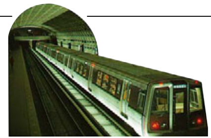
DRIVERLESS TRAINS? Most modern rapid transit systems, such as the Metro in Washington, D.C., are ideal for automation. This is because they have a steady flow of traffic and there is no disruption by slower freight trains or faster express services. The entire network is run by a central computer-based control system, and the trains need no motormen.
