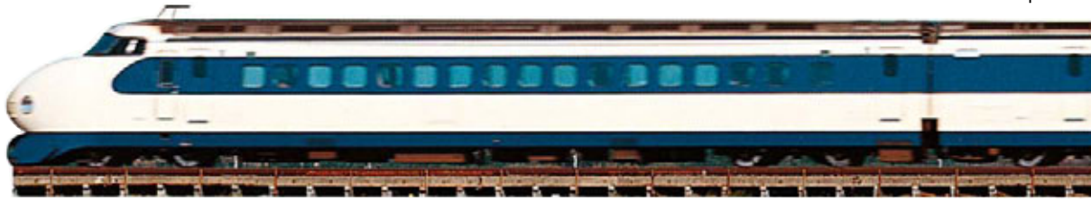
The first regular Shinkansen service, in 1965, traveled at an average speed of 101 mph (163 kph), with a maximum of 130 mph (210 kph)
