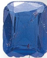
Chipped glass of a GTD
