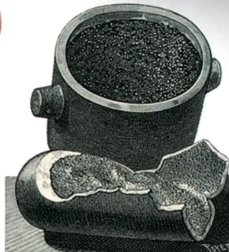
Two halves of synthetic ruby boule
