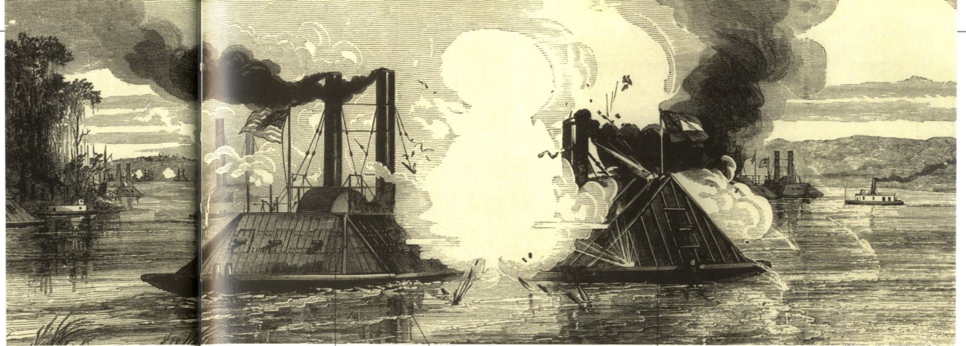
Iron plates, held on with rivets Armored paddle-wheel cover Sloping iron sides to deflect cannonballs
