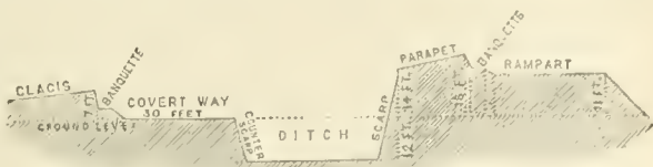
Vertical Section of Defence-works.
