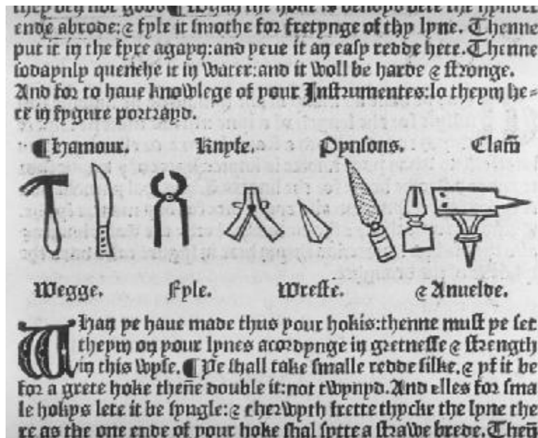
23.1 Instructions for a gentleman: tools used for making fishing tackle, illustrated in the Treatyse of fysshynge wyth an angle added to The booke of hawking, hunting and blasynge of arms in Wynkyn de Worde's edition of 1496.
