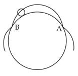
touches the circumference of the larger circle at the beginning and end of each revolution of the smaller circle thereupon, as at A and B in the figure. The curve A–B is the epicycloid. For instance, this figure shows the two circles: we will say that the point on the smaller circle begins its curve at A, rolling upwards to the left; at B, the point on the smaller circle has completed a full revolution; the curve A–B is the epicycloid.
