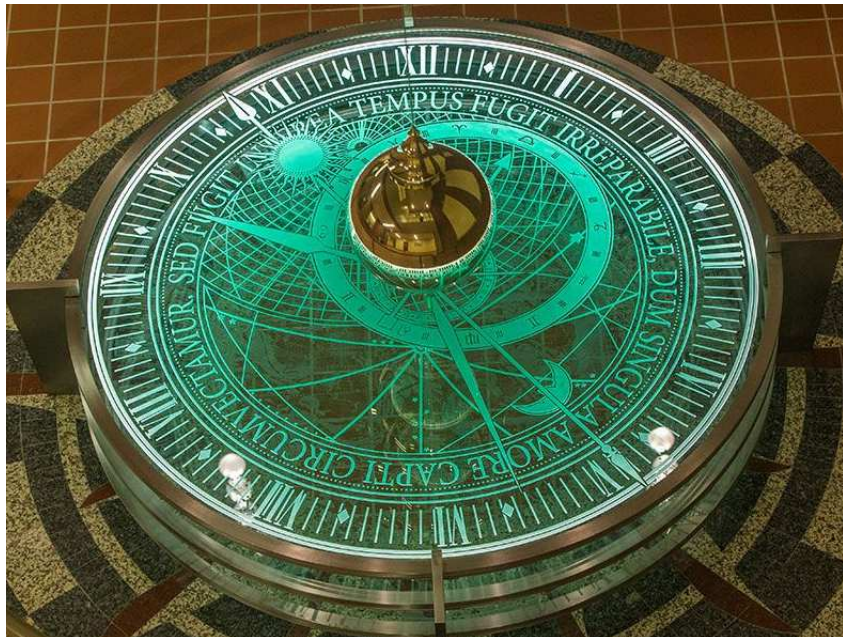
The Foucault Pendulum (above-shown version at the University of Miami) gives a very easy demonstration of the rotation of the Earth. Invented by French physicist Léon Foucault, it was first introduced in 1851 at the World's Fair in Paris. The Latin text translates as: Time flees irretrievably, while we wander around, prisoners of our love of detail. But meanwhile it flees.
