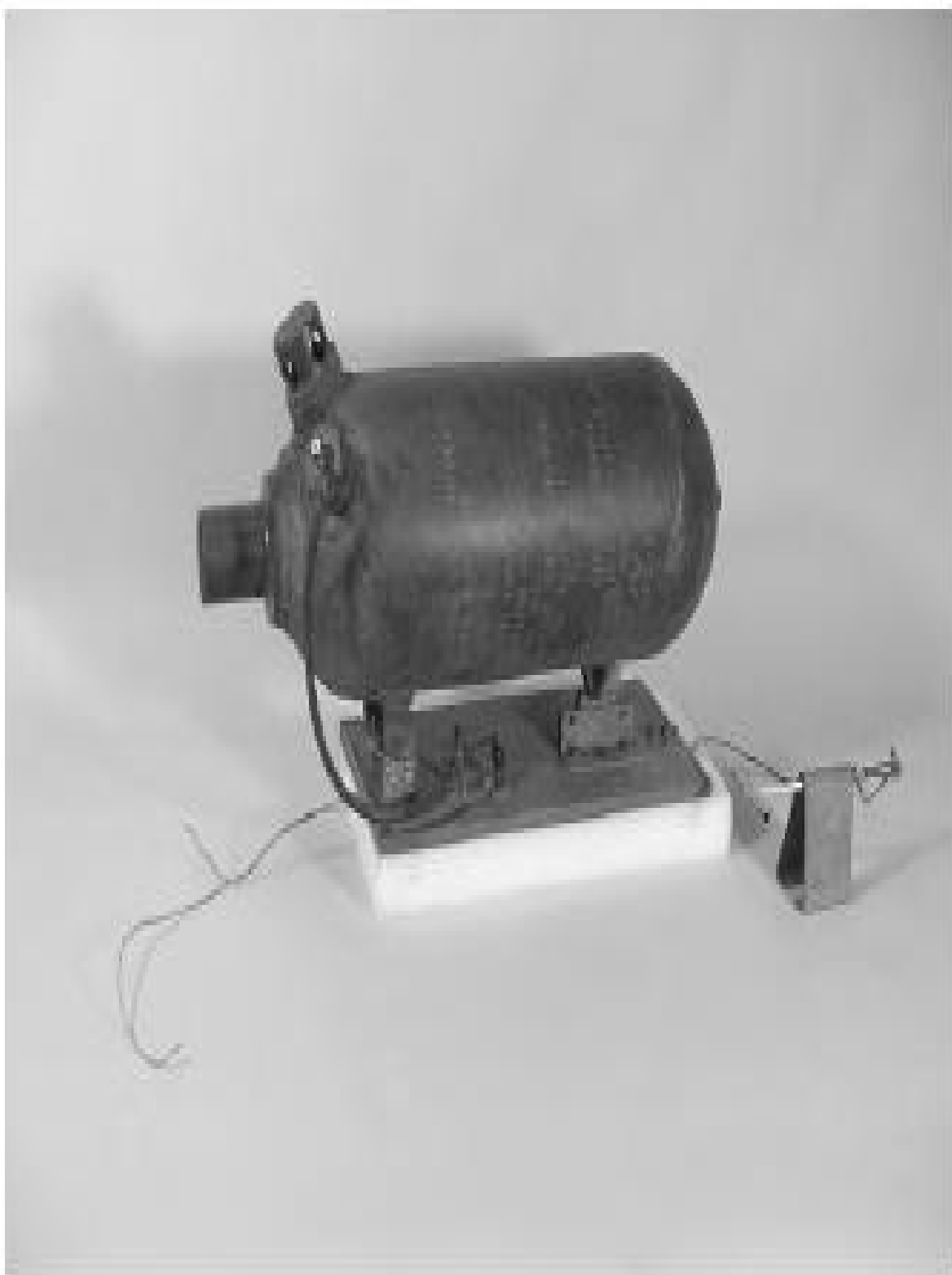
The JATO (Jet-Assisted Takeoff) rocket, a Jack Parsons invention (Aerojet).
