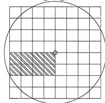
Ancient architects often wanted to *Square the Circle* to create a circular column of known cross section that could be set onto a square base. Their portable calculator for ‘Squaring the Circle’ was a simple 2 x 1 rectangular tablet. Draw a circle through one corner while centering on the corner diagonally opposite. The square has an area equal to 8 tablets.
