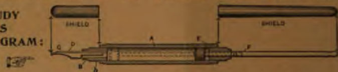
A, Barrel; B, Nozzle; C, Pen; D, Feed; E, Plunger; F, Rod.
