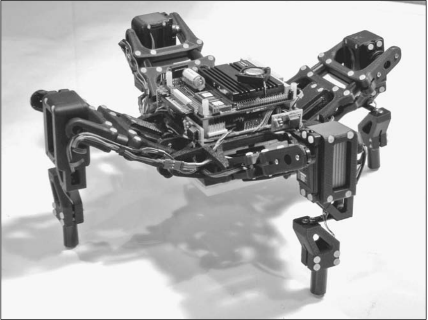
Figure 17a: Starfish, a four-legged robot that walks by using an internal self-model it has developed and which it continuously improves. If it loses a limb, it can adapt its internal self-model. 5
