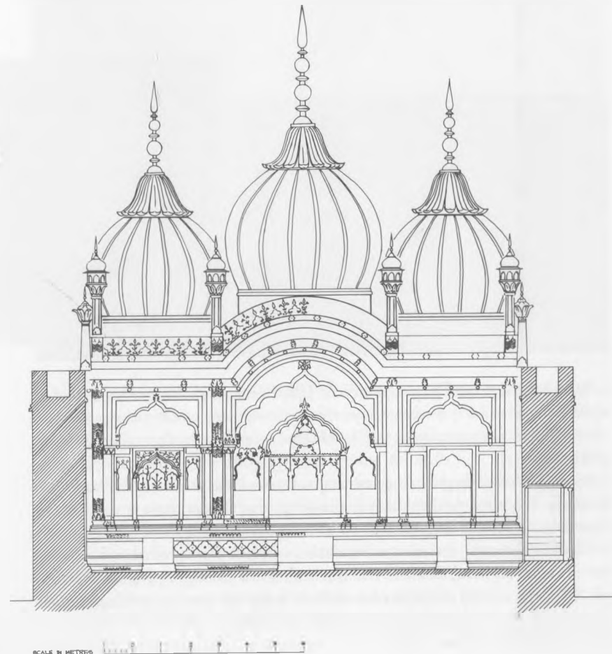
158 Delhi, Red Fort, Moti Masjid, 1663, elevation; the domes were rebuilt after the mutiny of 1857–58. (After Archaeological Survey of India)
