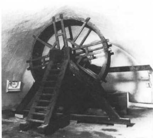
68 Treadwheel, for raising water from the well in Mont-Louis Citadel
