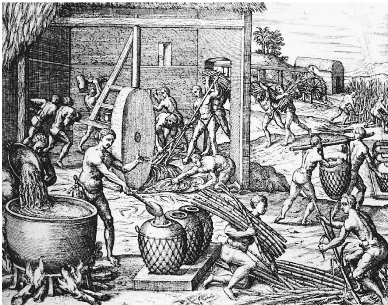
Sixteenth-Century Sugar Mill. This engraving, rendered in 1590 by Theodor de Bry, depicts the activities of Indian laborers at a New World sugar mill. The workers are shown cutting and hauling sugarcane, grinding it with a millstone, cooking the mash in a cauldron, and pouring syrup. LIBRARY OF CONGRESS.
