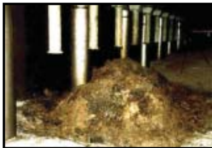
Pile of Lava-Produced Fuel-Containing Material in Bubble Room Area at Chernobyl
