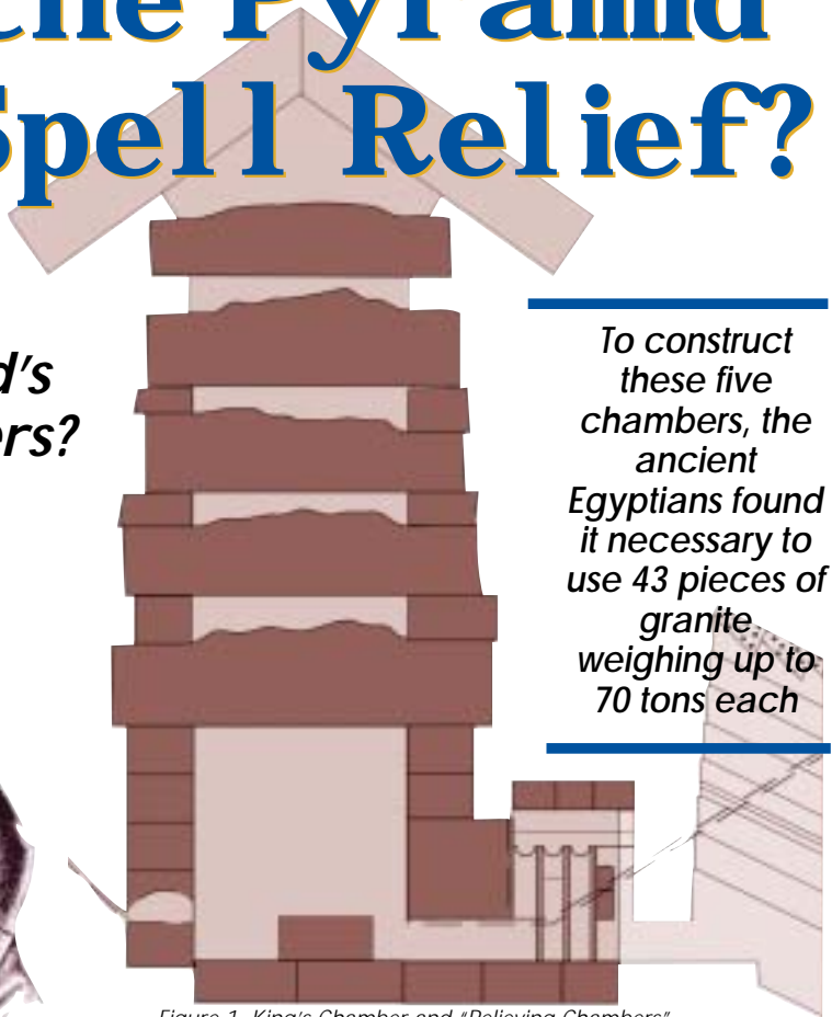
Figure 1. King's Chamber and "Relieving Chambers"
