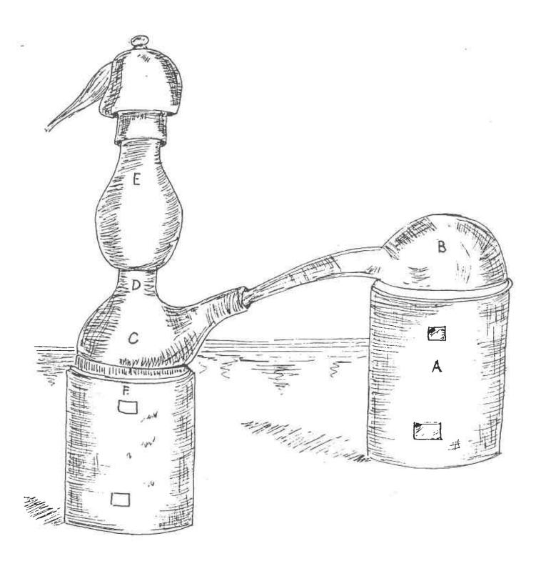
KIRKRINGIUS- A. is the Furnace, B. the Retort. C. the Recipient. D. the Aperture with a Pipe of a Moderate Bigness, on which may be set the Alembick E. The other Furnace is F. which containing a moderate Fire, sublimes what falls into the receiving Vessel up into the Alembick E. And so the Matter which is distilled from the Retort B., by the Fire of the Furnace F., is presently sublimed; which may not only be useful in this case, but also in every Sublimation of other Matters.
