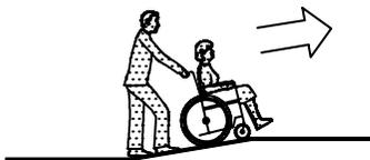
**c Ramp, 1:6 gradient, wheelchair user being pushed up**
