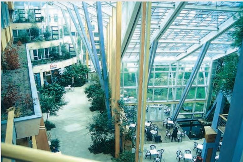
**All the glass sections in the roof can be opened to avoid overheating in Prismahuset, Nuremberg, Germany.**
