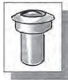
**Spark-arrester.** Sparks from the chimney flue and embers from wood ashes can cause fires. The sparks are made to rotate in a container where they are extinguished against the walls.
