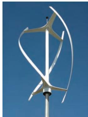
This helix-formed wind turbine has height 5m, diameter 3m and is adapted for mounting on building roofs.
