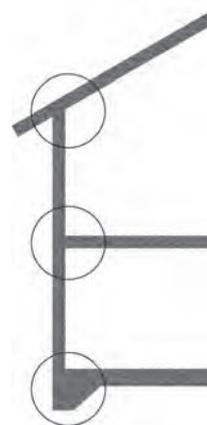
**Places where, in principle, thermal bridges can easily occur in a building if a structure is not well planned and built.**
