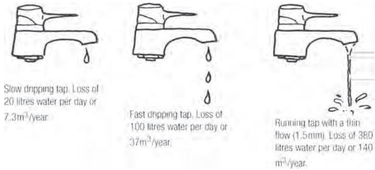
**Make sure that no taps or toilets drip or leak, which can quickly lead to large water losses. If it is hot water that is dripping, energy is also lost.**
