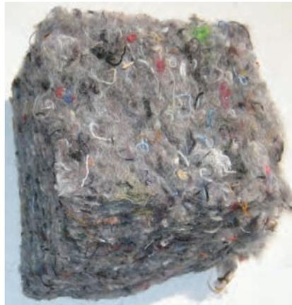
Textile fibre mats are made of textile waste and bound with plastic.
