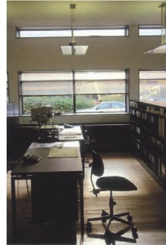
The main office of the Pihl & Sønner construction company in Copenhagen, Denmark, is naturally ventilated. Intake air is drawn through narrow, high slit windows that adjust automatically. The regular windows are opened and closed manually as required.
