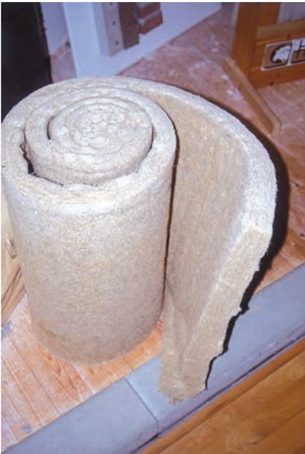
Flax fibre insulation in the form of a mat.
