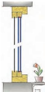
The inside glass is replaced with a double insulating argon-filled pane with soft-coated energy-efficient glass (if allowed by the construction of the casing). U-value: as low as  $1.3\text{W/m}^2\text{K}$ .
