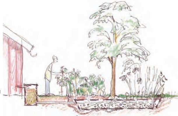
**A mull filter for treatment of water from bathing, dishwashing and clothes washing (greywater), before the water infiltrates into the ground.**
