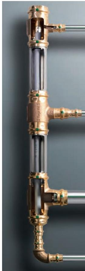
Viega Smartloop In Line System, a pipe-in-pipe system for shaft installations with the tap water circulation inside the hot water intake line using polybutylene piping. This results in less use of materials, less work hours, 20–30 per cent less heat loss, a smaller hot water pump, fewer tenders, and less installation.
