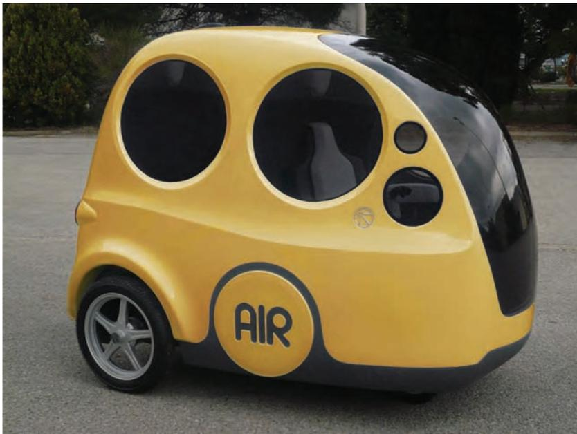
**The small French car Airpod is extremely cheap to operate. It runs on pressurized air, is 2m long and has enough space for three people. Top speed is 70km an hour and 100km can be driven on a tankful of pressurized air. It takes a couple of minutes to fill up the tank.**
