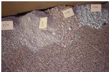
The various fractions of crushed concrete can be sorted according to size.
