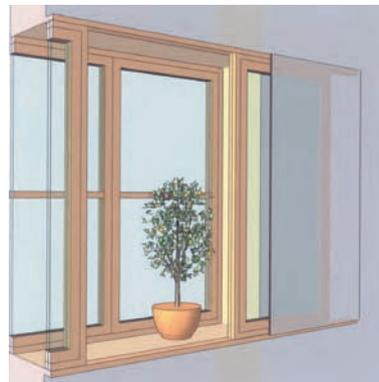
2+2-glazed method where during the summer the inside window slides into the wall or behind screens on the wall.
