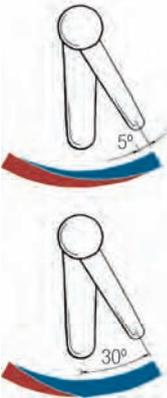
The figure above shows temperature zones for the different positions of a tap pointing sideways, and where the water is warm in the central position. The bottom figure shows the difference in temperature zones for a tap that runs cold instead of warm water when the lever is in the central and up position.
