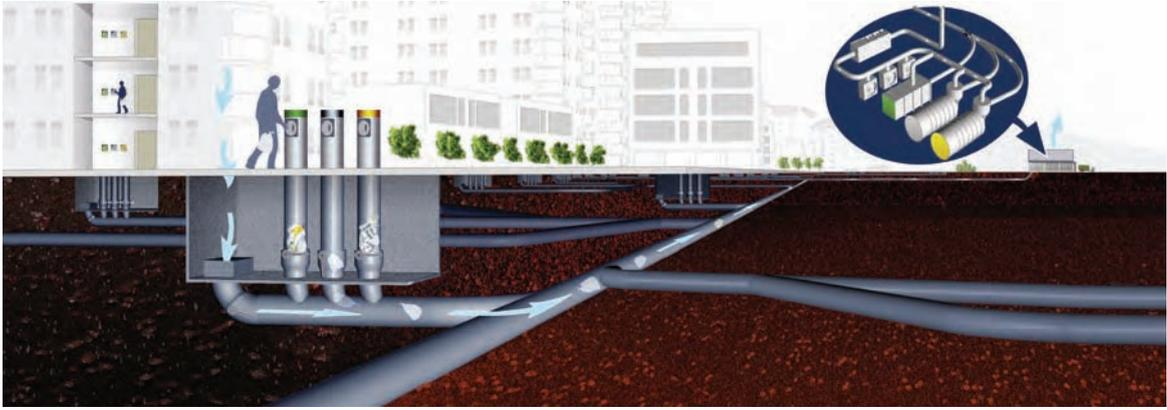
In Hammarby Sjöstad, Stockholm, there is an automated waste collection system from Envac. It consists of a fully enclosed vacuum system, doing away with foul-smelling, dirty refuse collection rooms and containers in the streets. No one needs to come into contact with refuse sacks or containers. Sorting at source is handled by using one inlet for each fraction: organic waste, paper and the rest.
