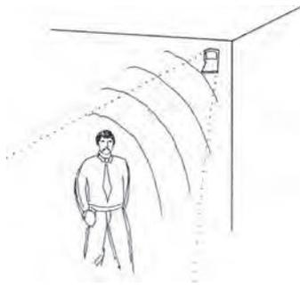
Motion detectors can be used to turn off lights in rooms that are not being used. Modern motion detectors sense heat and movement from people in a room. The latest ones react to sound/infrasound and the light dims on and off according to those. 75–95 per cent of the electricity can be saved in staircase and garage lighting etc.
