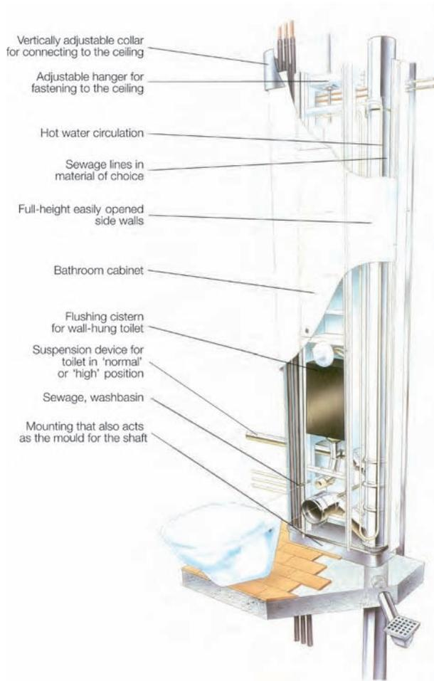
**A wet area wall can be purchased incorporating a cassette with outlet pipes for cold water, hot water, and toilet and circulation.**
