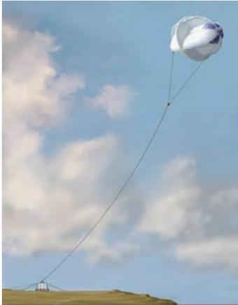
The Canadian company Magenn has developed a system where a large helium balloon twists around in the air which generates electricity via the cable it is anchored to.
