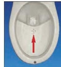
**The German urine-separating vacuum toilet Ro-evac No Mix Toilet from Roedinger. The toilet bowl has two outlets, urine runs down the front outlet and is transported away undiluted, faecal matter falls down the back outlet. As soon as the toilet is flushed, the cover over the urine outlet closes.**
