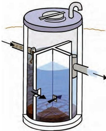
**Sludge separation can take place efficiently in a three-compartment septic tank made of concrete. Most modern sludge separators are made of plastic.**
