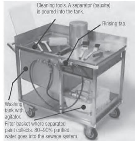
The paint company Beckers's wash cart with a paint separator provides an on-site solution for the environmental problems arising when paint-brushes are washed. The cart was developed by master painter Alf Karlsson.
