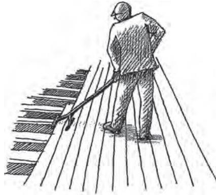
**For removal of floor boards, wallboards and tongue-and-groove ceiling boards, there is a special-purpose crowbar available that allows a lot of force to be used without damaging the boards. These crowbars are available in different sizes to suit various types of timber.**
