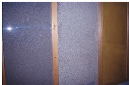
Cellulose fibre is in the compartment on the left, perlite is in the middle and on the right is mineral wool.
