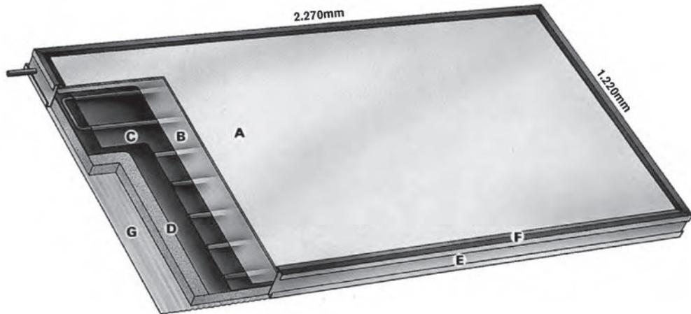
In Sweden, flat-plate solar collectors are most common. The illustration shows the construction of a TeknoTerm collector.
