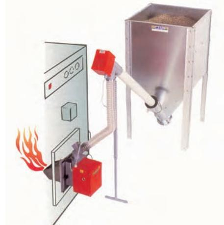
In small properties a pellet burner often replaces an oil burner. The burner is integrated with a storage silo filled with pellets. The silo can be placed 5–10m from the burner if necessary.
