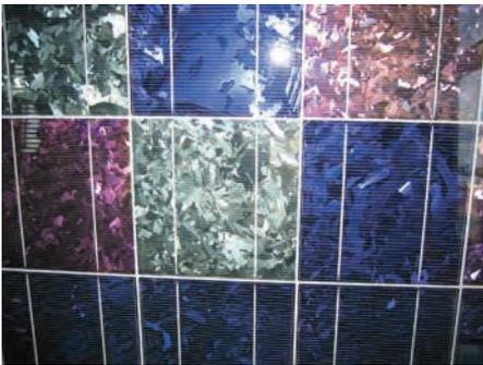
Different types of solar cells vary in colour, level of efficiency and other characteristics. Polycrystalline cells' colour varies a lot, while CIGS cells are naturally completely black.
