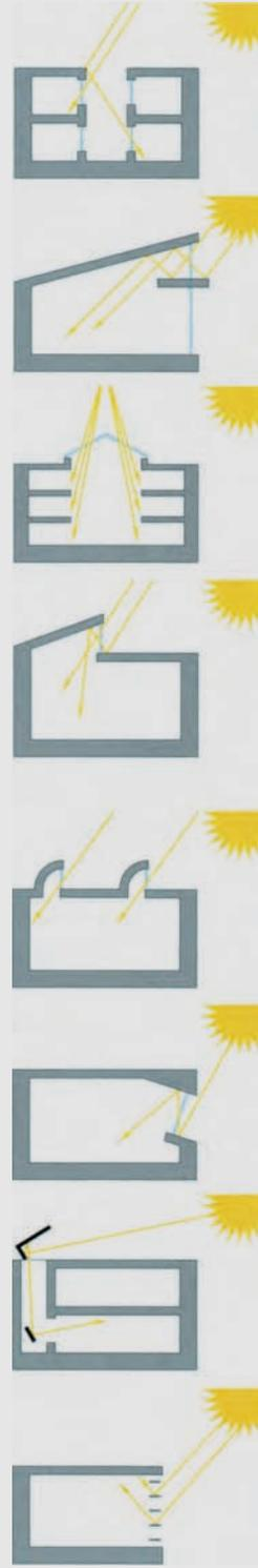
**Different principles for making use of daylight.**
