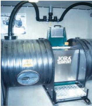
In a drum composter, waste is put into one end of a drum and eventually comes out the other end as composted waste. The drum inclines and slowly rotates, or is equipped with a mixer that pushes the material forward in the drum.
