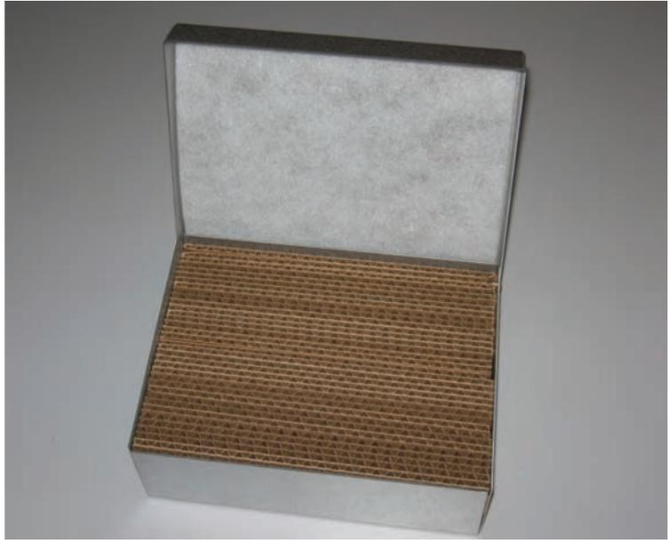
**Air Star is a decentralized ventilation system with a unit in each room. It alternately conveys in fresh air, which is heated by the heat exchanger, and conveys out air that heats up the heat exchanger. The heat exchanger is made up of corrugated cardboard and stores that heat through sorption. Water is gathered from the moisture in the exhaust air and absorption and condensation heat is created.**
