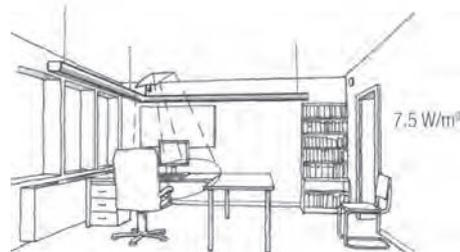
**Development of energy-efficient lighting has progressed quickly. Energy-efficient light sources, electronic control devices, fixtures and better planning for lighting are now available. It was formerly common for offices to use 45W/m<sup>2</sup>. Today, 15W/m<sup>2</sup> is used to manage the same light conditions. Today's technology can satisfy the requirements with 7.5W/m<sup>2</sup>.**
