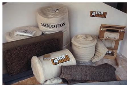
Insulating materials for sale at an ecoconstruction products exhibition in Germany. Shown here are insulation materials made of wool, flax and cotton.
