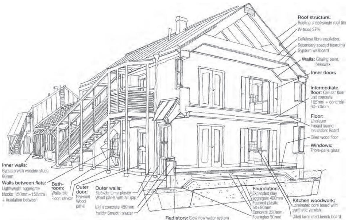
The Sjö district of Vadstena, Sweden (Erik Asmussen, architect) is built using 45cm-thick solid lightweight concrete. A homogeneous, relatively heavy wall was wanted, and lightweight concrete was chosen despite its low insulation value. The roof structure is insulated with cellulose fibre and there is foam glass under the ground slab.
