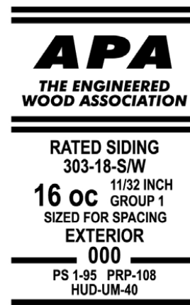
FIGURE 7.1 Wall siding grade stamp. (Courtesy of APA—The Engineered Wood Association, Tacoma, WA.)
