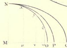
Figure 3.—Plan of a polygonal dome, showing the covering extended, and the angle-rib. The method of finding the covering and angle-rib for Figures 2 and 3, is the same as in Figure 1, and may be described in the same words.
