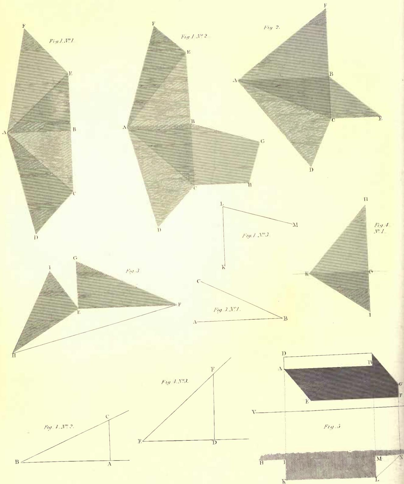
representations, the object is represented upon two planes, one parallel, and the other perpendicular to the horizon.
