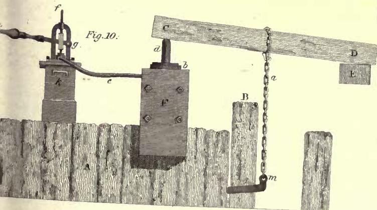
*Section of Valves Pile Engine.*
