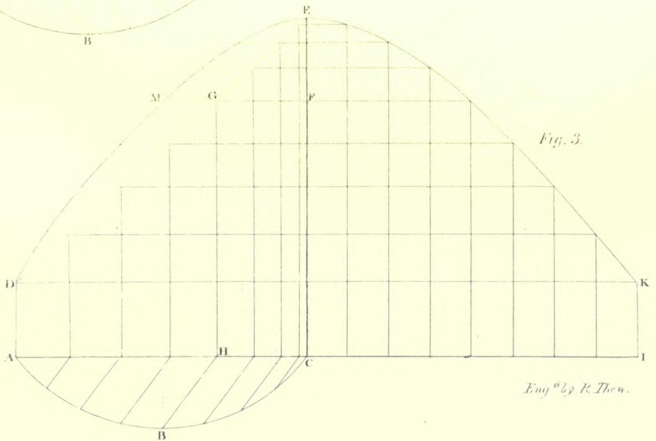
circle in the same plane, so that in each circle, the distance between the point of contact at the commencement of the motion, and the point of contact at any instant while in motion, is equal one to the other. Hence if the circumferences are equal, all parts of the circumference of the moving circle will have been in contact with all the parts of the circumference of the quiescent circle.
