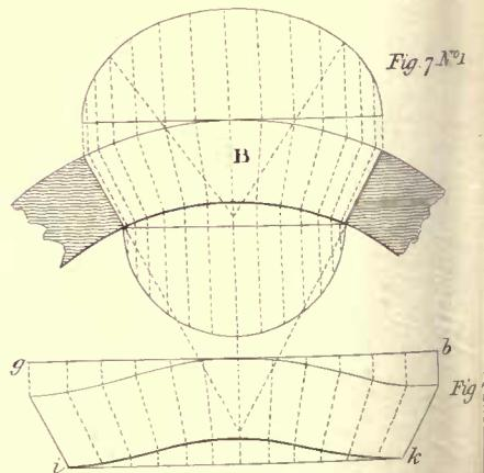
number of equal parts, the more the truer the work, and run these parts on the dotted arch-line figure; then draw a line from *a* to *g*, which is the soffit stretched out; then draw a dotted line from the centre, *a*, the parts of the arch-line, stretched out far enough to receive the parts taken from the chord-line to the inside of the wall, and set them on the soffit, stretched out, as 1, 2, 3, 4, 5, 6, 7, 8, and so on; which will give the edge of the soffit.
