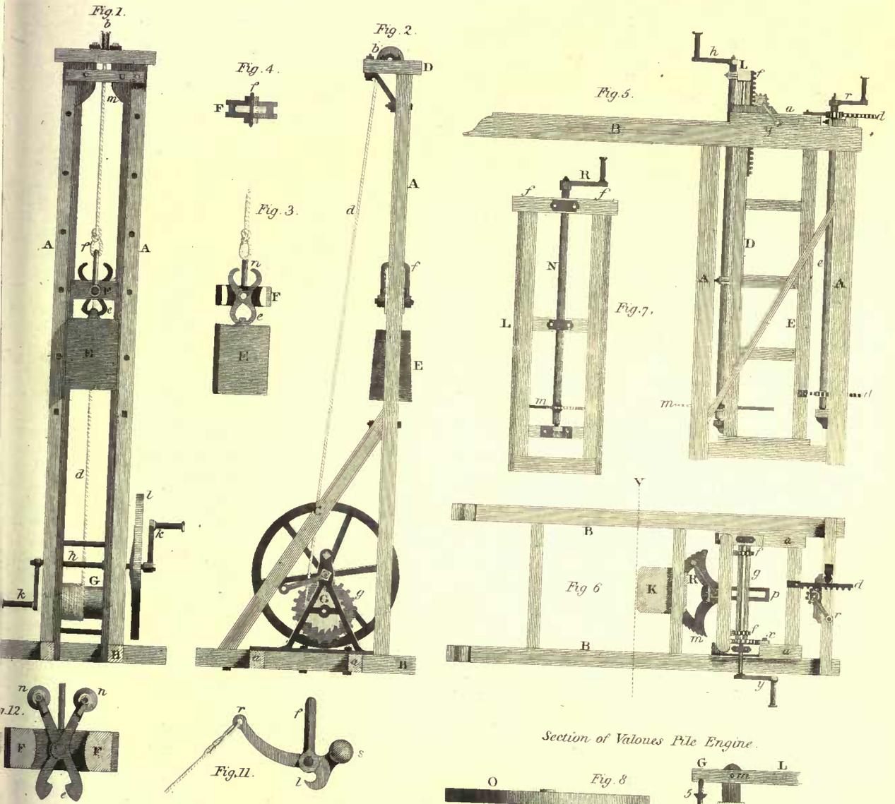
*M. Bramah's Machine for Drawing Piles out of the Ground.*
