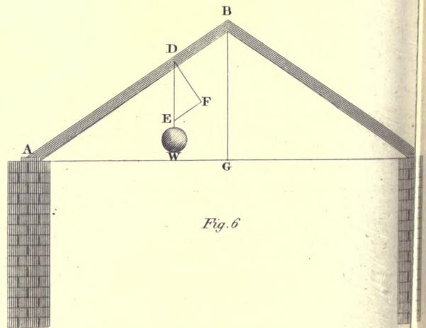
to the horizon, these lines being produced, they may be supposed to meet at an infinite distance. To find the pressure on the walls: join  $DC$ , and produce the vertical line,  $KG$ , to meet it in  $E$ ; then, if  $G$  be supposed to be the weight of the body, the pressure on  $D$  will be  $\frac{EC \times G}{DC}$ , and the pressure
