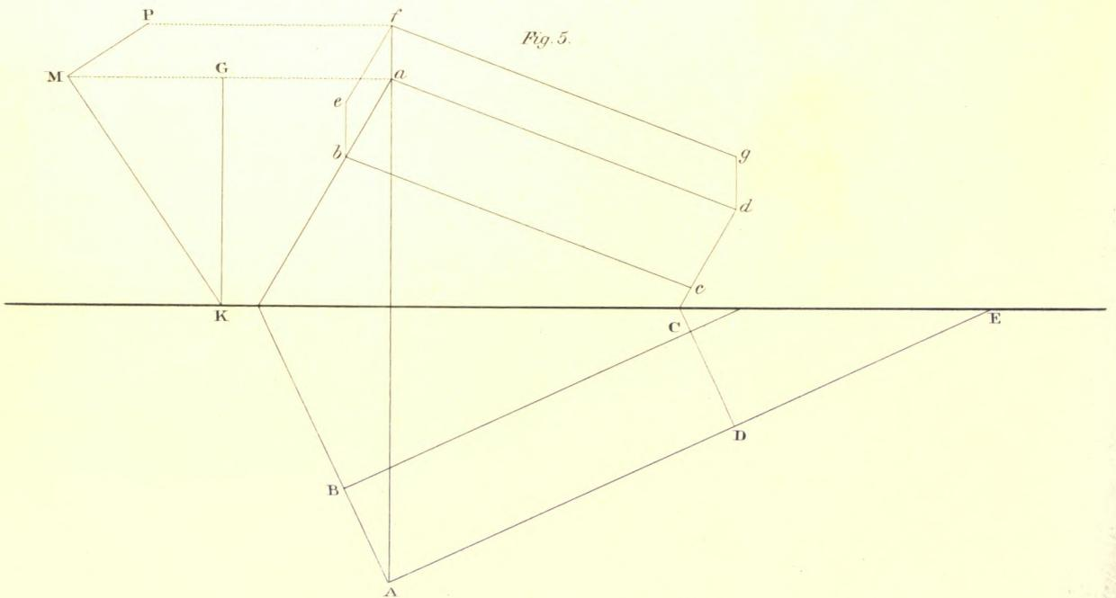
ellipsoid  $b c d e$ . This may be done as in Problem I., Method V. of the article ELLIPSIS (Vol. I., page 365), or by finding the two axes, as in Method I., (page 365), of the same article.
