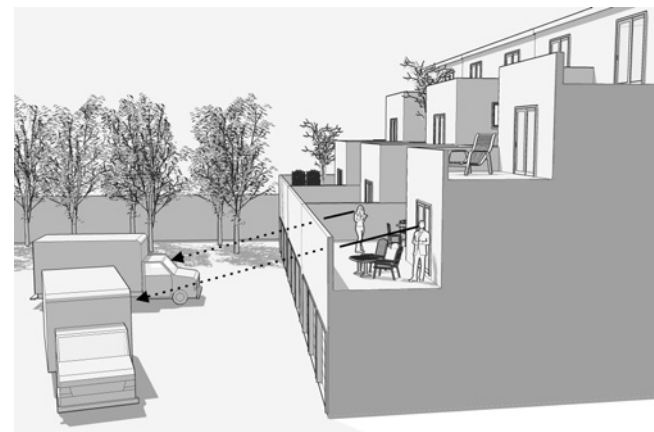
Figure 6.34 Try and find ways to reduce the impact of service areas on views from homes
