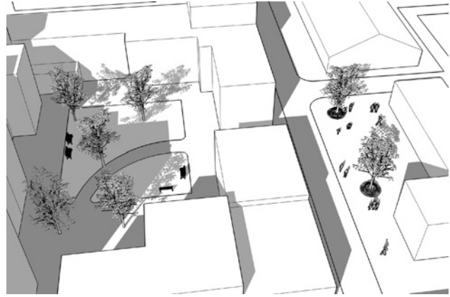
Figure 9.9 In temperate climates ensure that outdoor spaces get access to the sun
