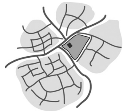
Figure 6.22 More recent new urbanist thinking has put the school on the edge of neighbourhoods so that they can be shared and the playing fields don't divide the communities
