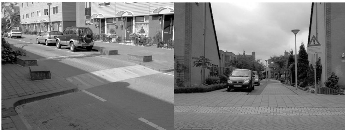
Figure 5.46 Vertical traffic calming measures
