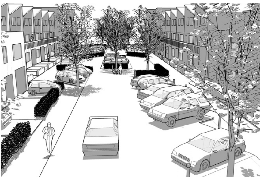
Figure 9.39 Parking, trees and other features might be used to limit significant views to encourage a slower driving speed
