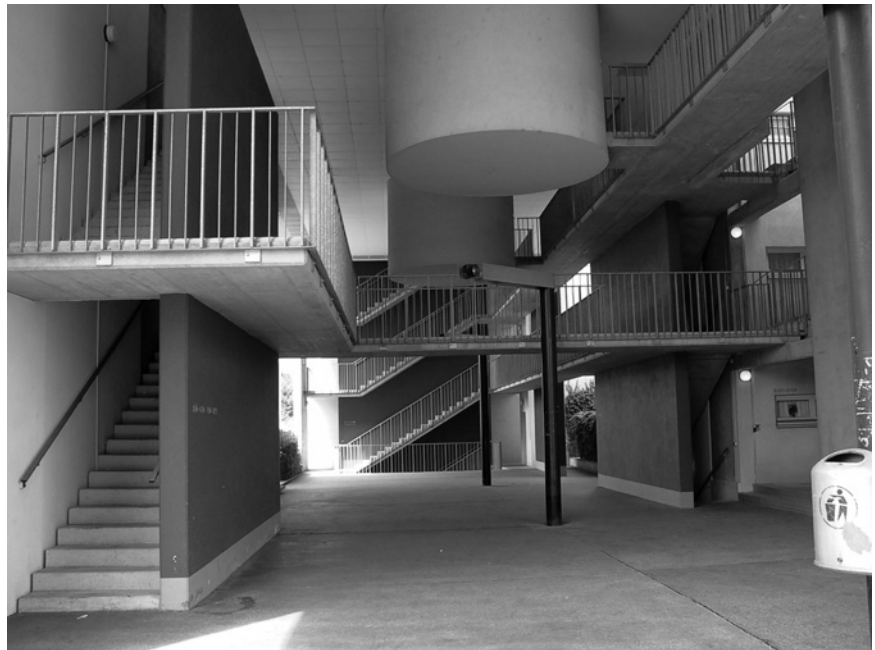
Figure 7.41 Comprehensive deck access developments tend to create depressing, insecure and inconvenient pedestrian environments leaving the ground floor to become dominated by traffic
