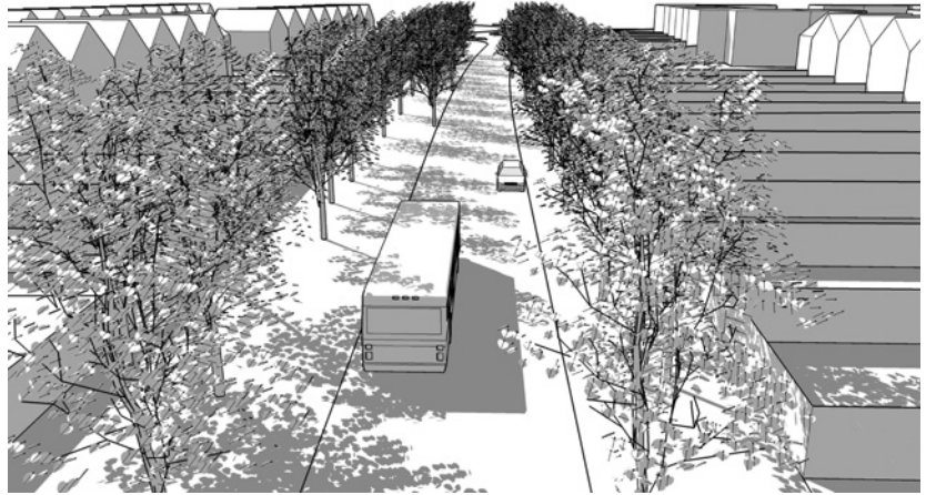
Figure 7.42 Principal access roads dominated by landscaping can be disorientating
