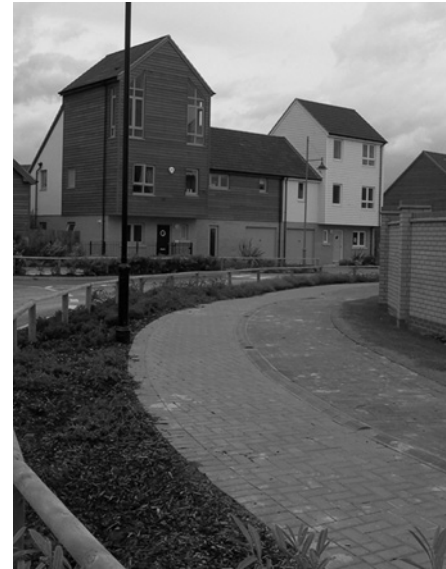
Figure 5.32 Cycle lanes might be highlighted with a change of material or colour
