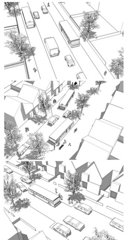
Figure 4.27 Provision of bus lanes and stopping bays should vary according to the status of the route
