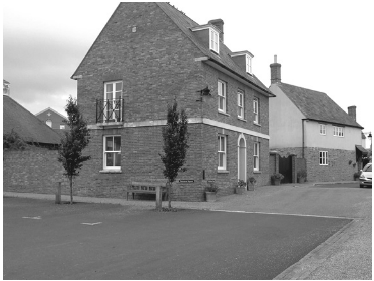
Figure 5.49 Tight corners slow down vehicles, but so does putting a building directly onto a corner to reduce the opportunity for a driver to see passing traffic until the point that the junction is reached
