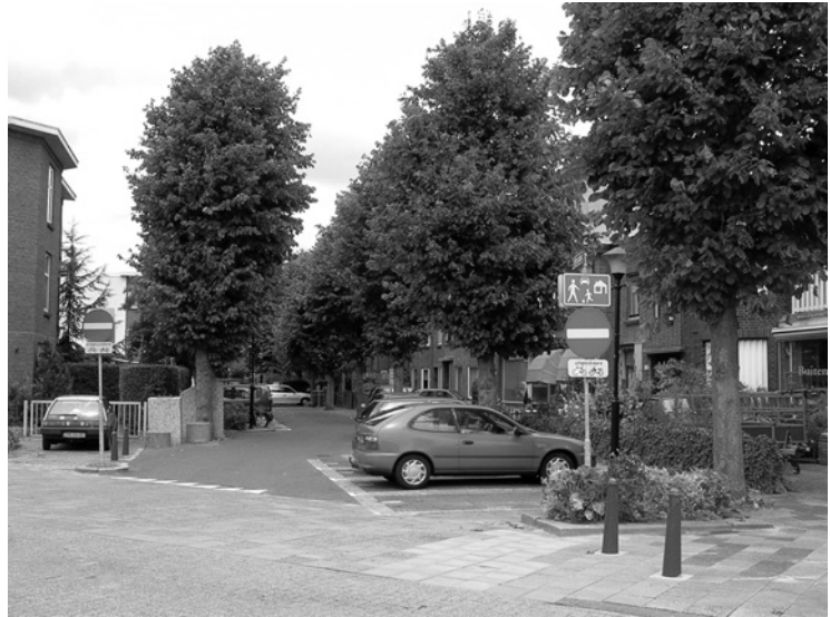
Figure 5.22 A combination of traffic calming techniques produces an environment where vehicular access is possible but only at a very slow speed
