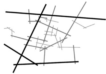
Figure 6.10 Illustration of an axial map produced as a result of space syntax analysis and based on Hillier (1996, Figure 4.7c). The darker routes are the most integrated and would be the better locations for uses requiring passing trade
