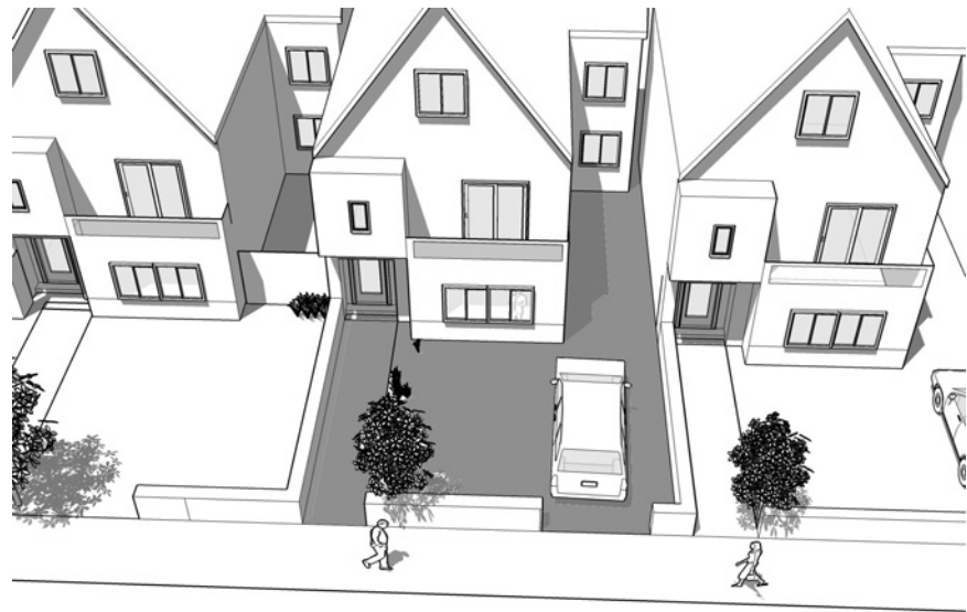
Figure 7.8 The shaded area highlights the area of semi-private defensible space in front of the traditional house on the street that residents find easy to control
