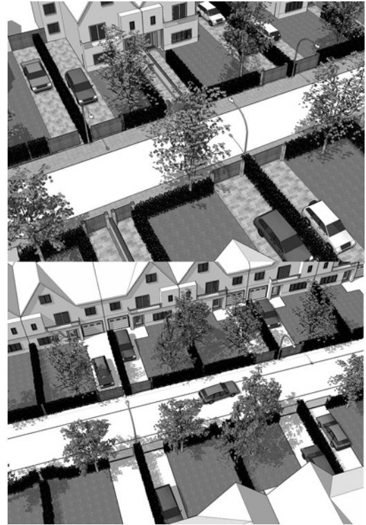
Figure 8.47 Grouped gardens, paths and drives (bottom) might extend the garden frontage within the street
