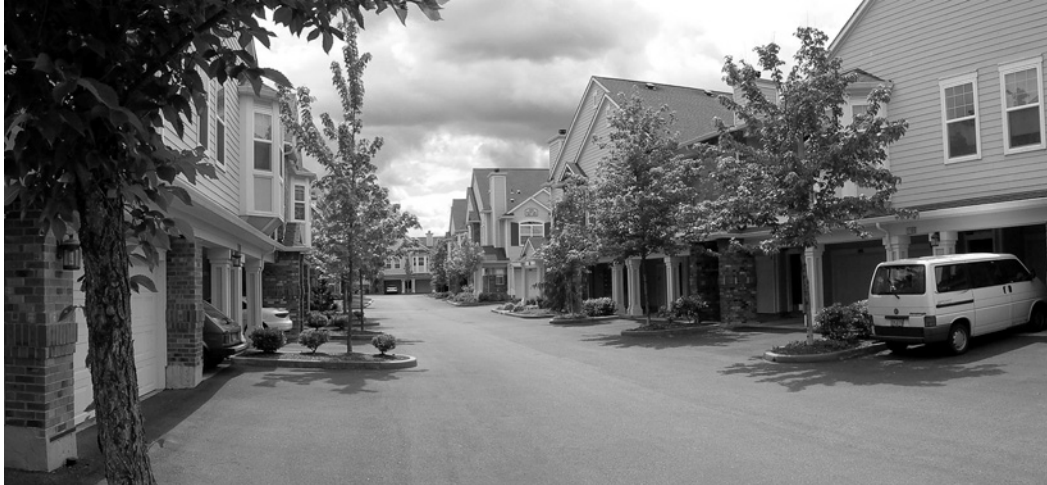
Figure 4.12 Where houses back the pavement any trees should be introduced into the street space
