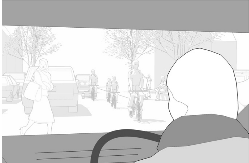
Figure 9.1 Streets should be designed so that people mediate their way through the space by using direct eye contact with each other
