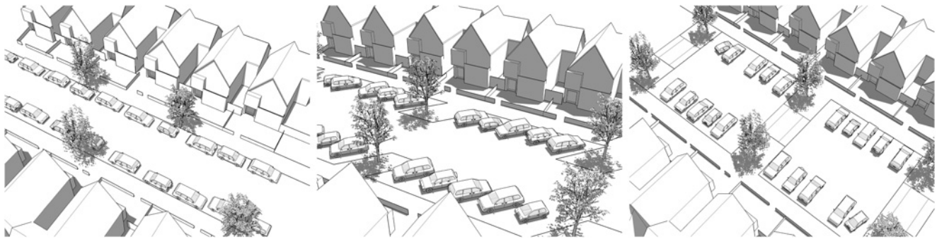
Figure 5.65(a) Parallel on-street parking
