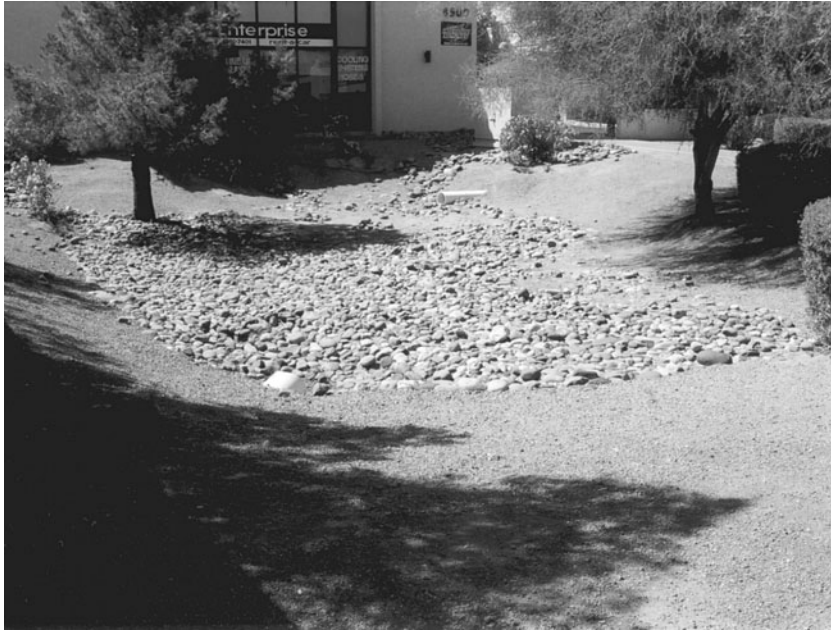
Figure 10.4 Small space treatment of runoff.
