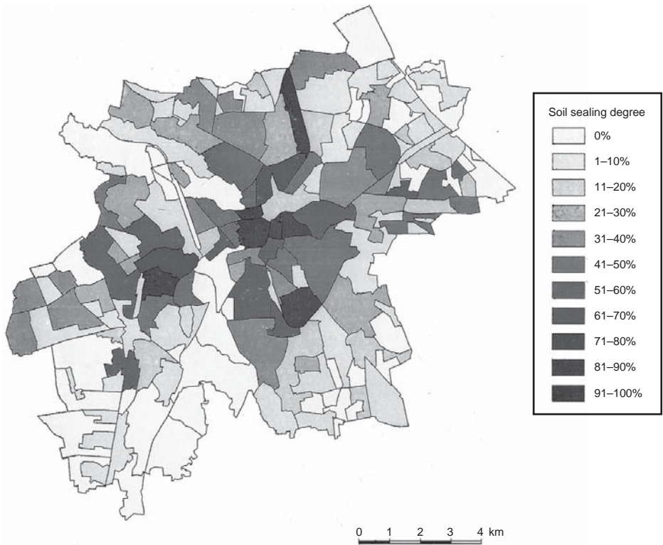
Fig. 21.4. Soil sealing map of Leipzig, Germany (in 10% classes) (Kabisch et al. , 1997). See also colour plate.
