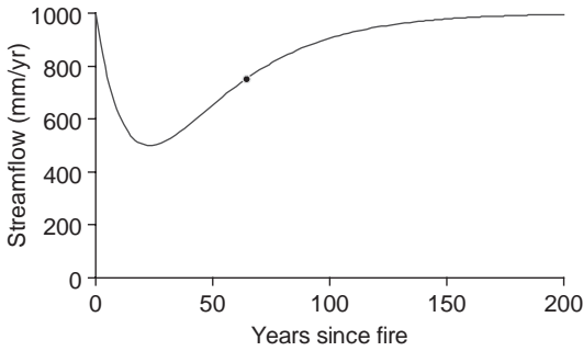
Fig. 7.2. Predicted streamflow per year from mountain ash forest as a function of forest age (based on Kuczera, 1987). The dot represents the age in 2004 of much of the mountain ash forest that was burnt in 1939.
