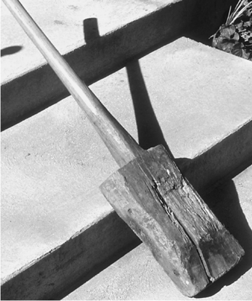
5-3. A wooden tamper used to compact mud in pisé construction in northern Peru (photo by the author, 1985).
