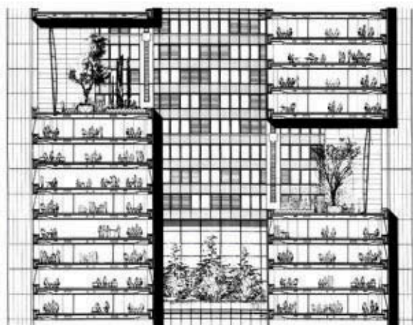
11.2 Section through the Commerzbank in Frankfurt showing the relationship between the atrium, sky gardens and offices
