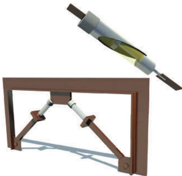
14.2 Visco-elastic damping distributed across multiple locations enabling redundancy and hence reliability for ULS design
