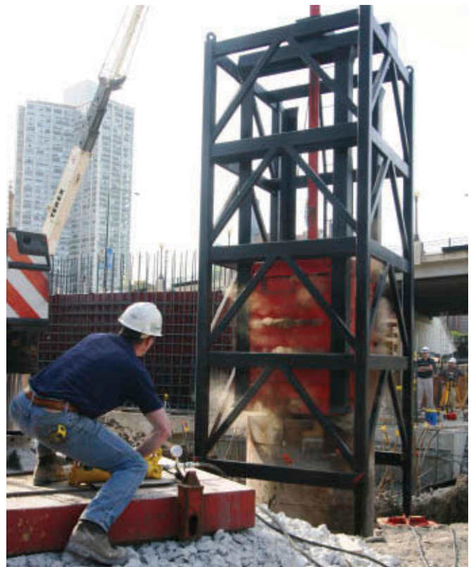
18.5 Large-strain dynamic load test (Apple 4) on a 2-meter diameter bored pile in Chicago
