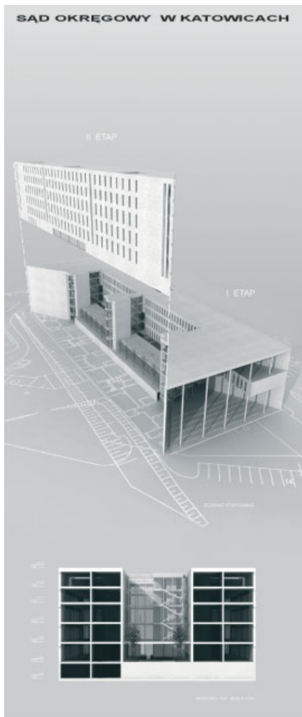
Exploded isometric (above, with part plan) and cross section (below). The composition and assembly of the building is necessarily simple, yet within a straightforward diagram the design manages to satisfy the complex spatial and circulation requirements of the programme.
