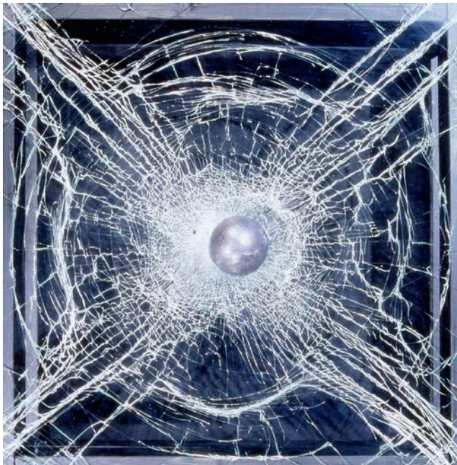
Illustration 7.52 "From Fracture to Form" (1996). Glass fracture pattern from the impact of a cannonball allows for a visualization of the multi-directional load-sharing behavior of edge-supported slabs. From an experiment at AHO by Arne P. Eggen and Nils E. Forsén. Photographer: Jiri Havran.
