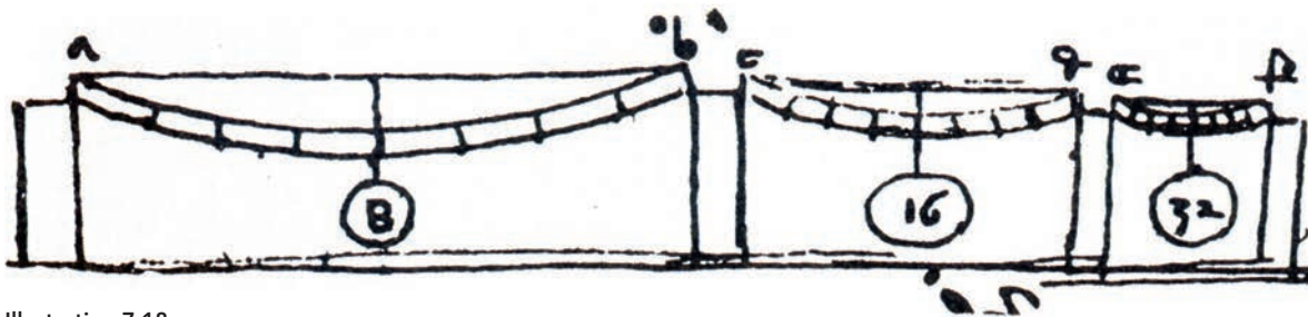
Illustration 7.18 Leonardo da Vinci’s diagrams of relative deflections for various beam spans.
