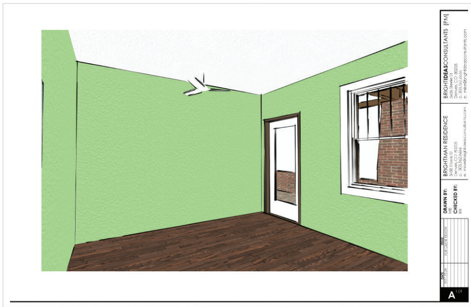
Figure 10.23 The Raster rendering setting is best utilized on viewports with complex styles and texture images.
