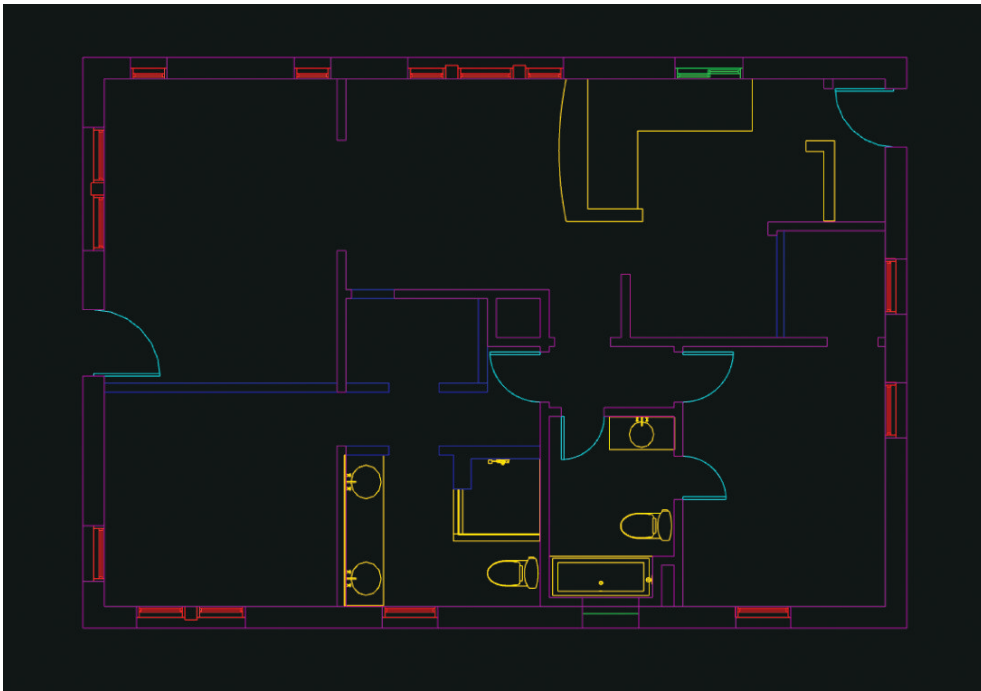
Figure 18.13 This proposed plan was created by referencing several .dwg exports from SketchUp into a 2D CAD program. Each .dwg reference is on a different colored layer, each different color represents the possibility for varying line weights.
