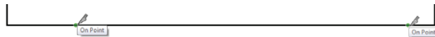
Figure 13.29 The Split tool breaks lines into separate segments, which can have different Shape Style properties.
