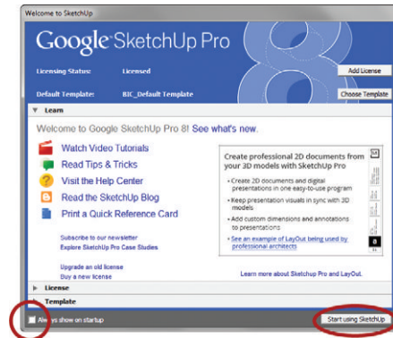
Figure 5.1 The Welcome to SketchUp Window offers links to learning resources, licensing information, and the default template. All of this information and more is available in the Help menu and at SketchUp.com.
