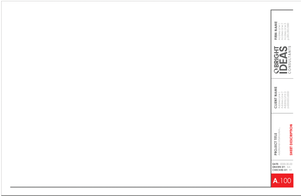
Figure 13.8 Assign red entities to the ANNOTATIONS layer. Assign gray entities to the TITLE BLOCK layer.
